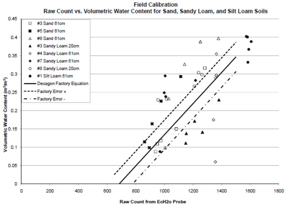
Figure 4. Field Calibration Compared to Factory Calibration Curve for Sand, Sandy Loam, and Silt Loam Soils
