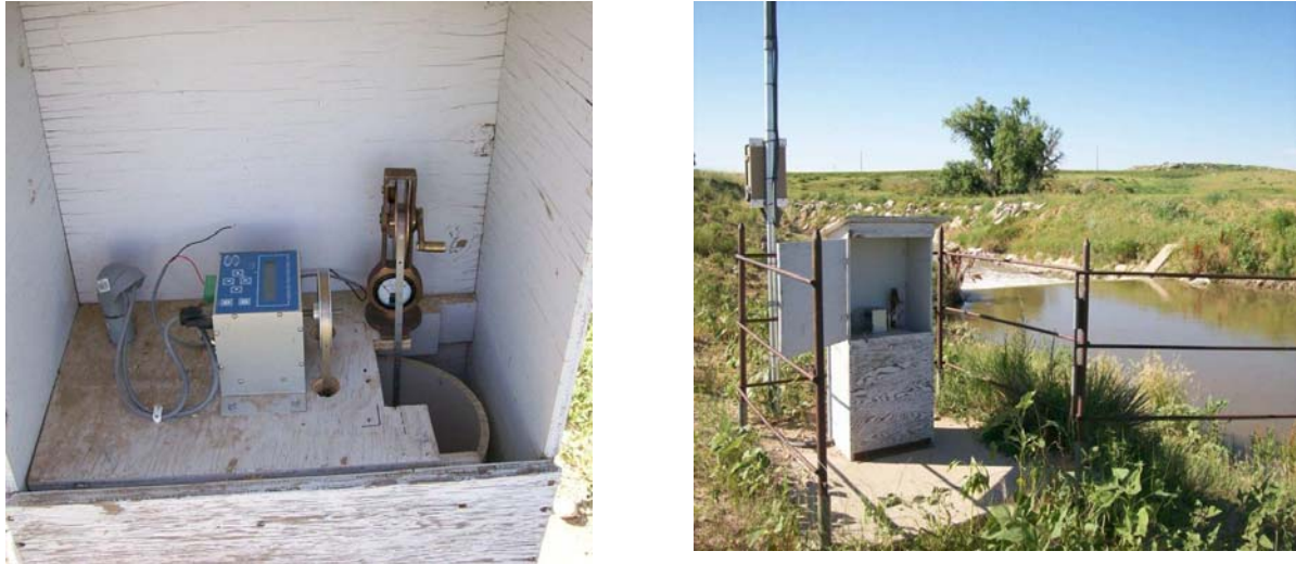
Figure 5. Cooperative Program SDR/cell phone telemetry streamgage.
