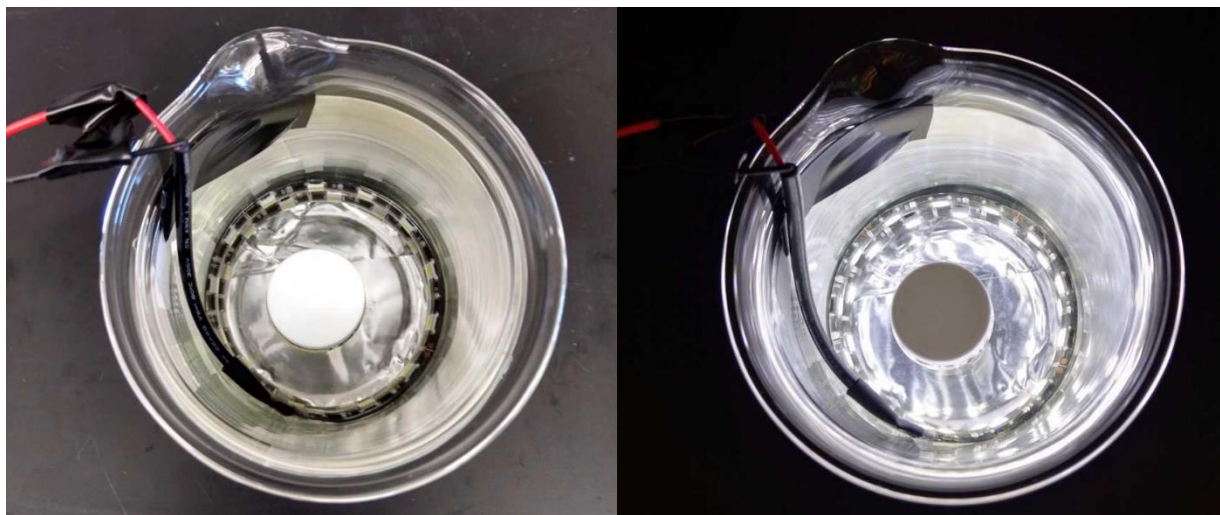
Figure 3.6: LED beaker photoreactors shown off (left) and on (right).
