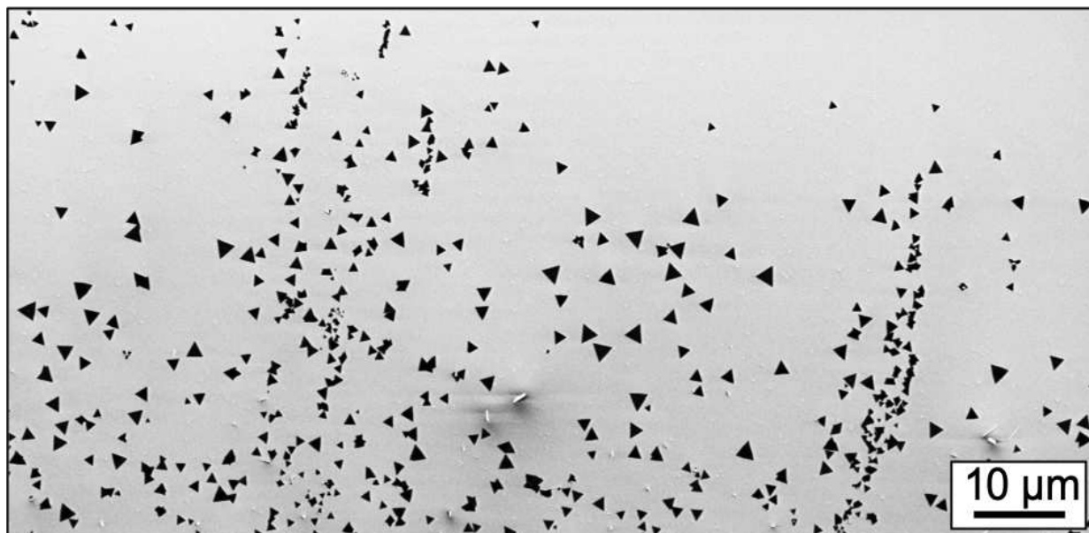
Figure 5: SEM image of triangular morphologies from the initial reaction conditions. The \text{MoO}_3 and S precursors were placed 16.0 cm apart. The pressure was held at 710 torr throughout the reaction. The maximum temperature used was 800 ^\circ\text{C} , for the 15 min hold time reaction.
