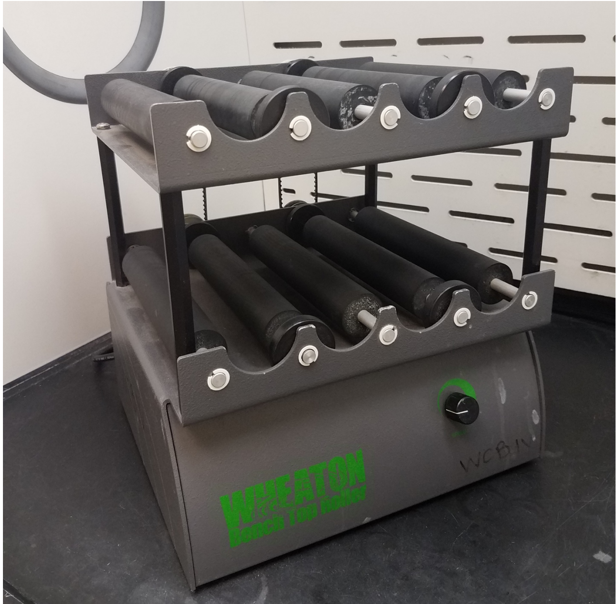
Figure 2.4: Picture of Wheaton Bench Top Roller used to prepare bottles for bottle assay. Bottles were laid on their sides on the rollers and were allowed to rotate to evenly distribute permethrin solution within bottle interiors. Photo by Ashley Janich.
