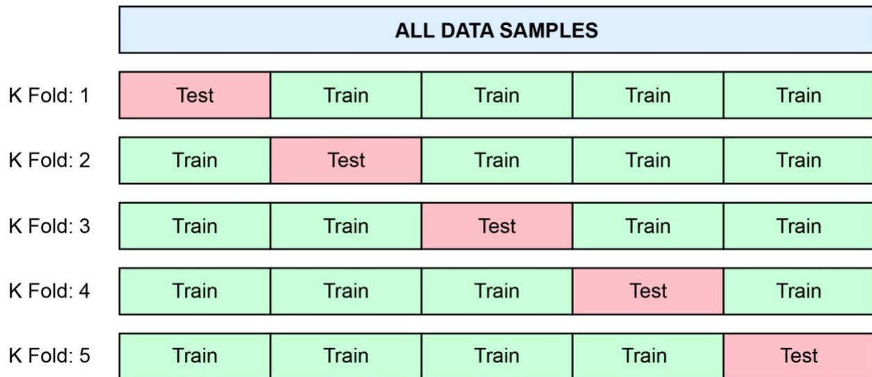
Figure 10. K-fold ( k = 5 ) cross-validation. All data samples are split into five different folds. In each fold, the machine learning algorithm is trained on four of the folds and is tested on the remaining fold. The overall performance of the algorithm is calculated by averaging the results of the test folds.
