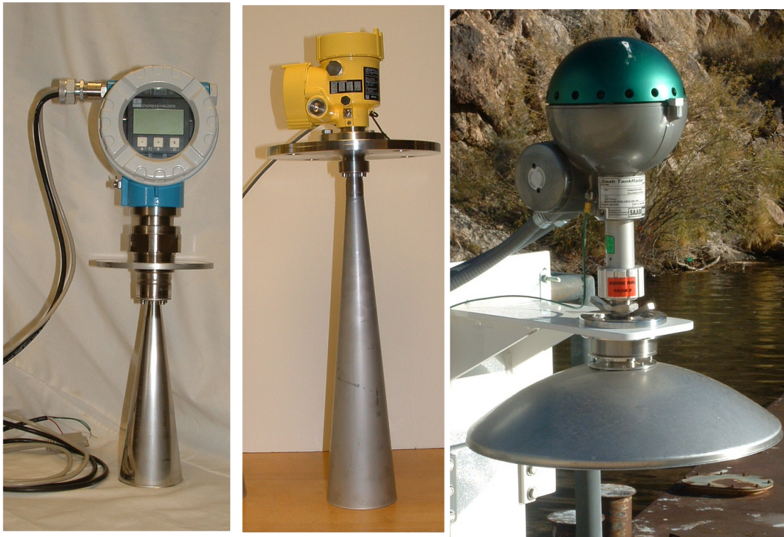
Figure 1. Pictured from left to right, Design Analysis Associates H-3611, Ohmart Vega Puls 62 and Saab Rosemount Tank Radar. Photos are not to scale.
