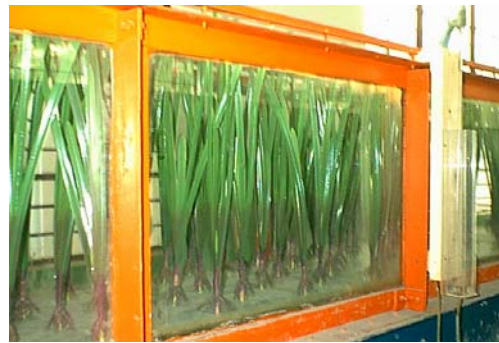
Figure 3. Experimental facilities for vegetated-bed test.
