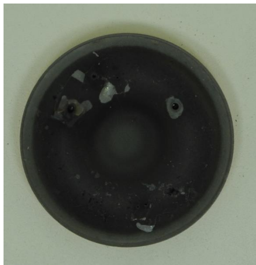
Figure 25: ZnTe sputtering target after charge buildup on the surface.
