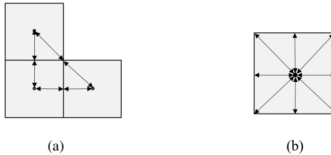
Fig. 3. (a). Each link is split into two segments. (b). The eight link segments connect to a node.
