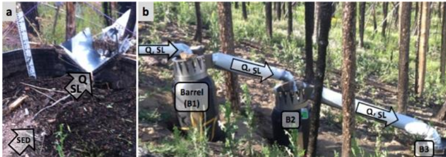
Figure 4.2. Hillslope runoff and erosion monitoring: (a) sediment fence in the foreground captures sediment (SED), and a 90° V-notch weir routes runoff (Q) and suspended load (SL) into a series of three collection barrels; (b) side view of the Q and SL collection system with sample collection barrels labeled sequentially as B1-B3. Note the staff gauge in panel a, which was used alongside a time lapse camera (upslope, not pictured) to determine the height of water above the weir at 1-min intervals for use in equation 4.2.
