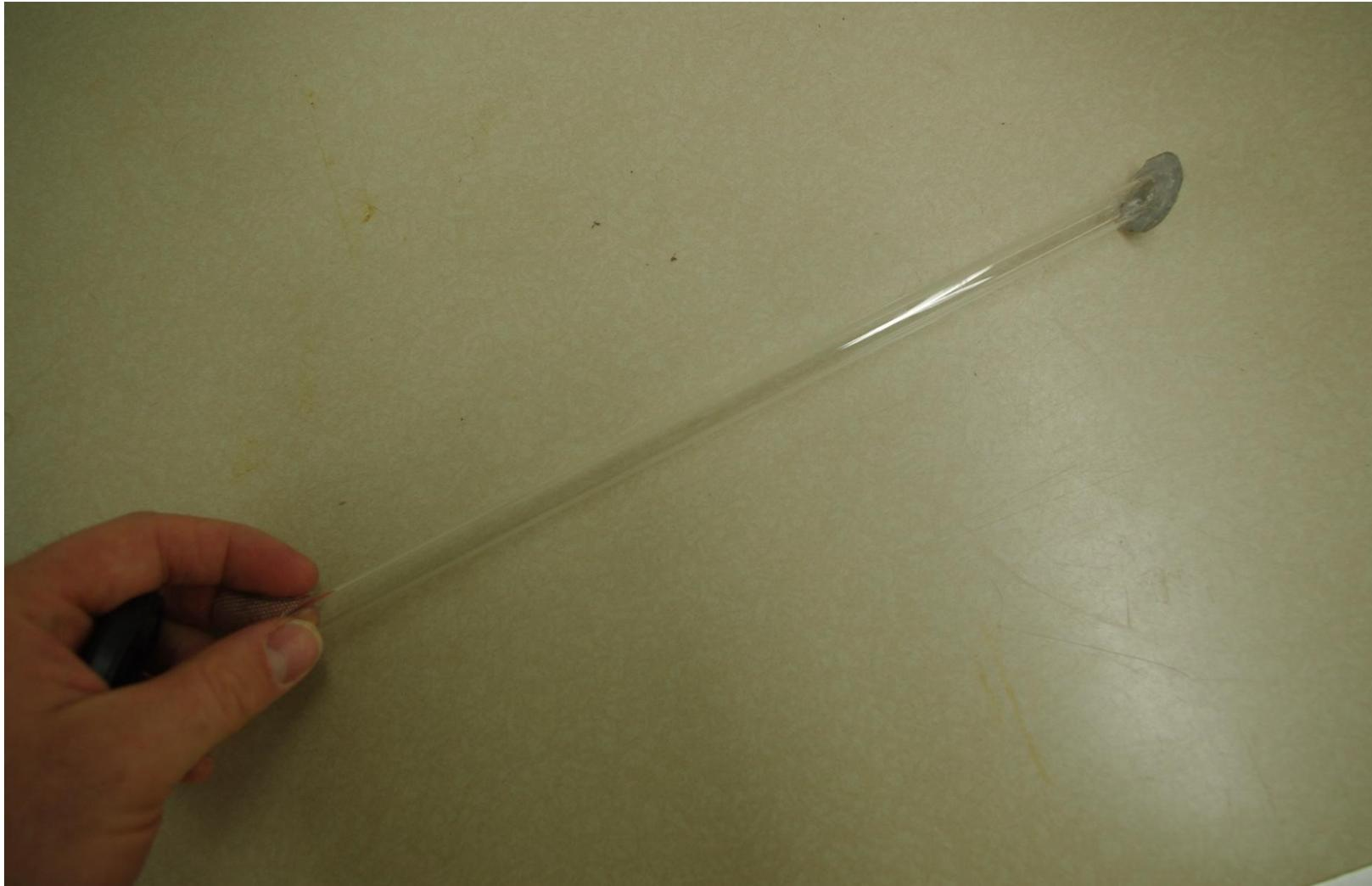
Figure 4.S2 - Exposure tubes. Aquarium-grade silicone was used to affix stainless steel mesh (105 x 125 micron pore size) to the beveled (30°) end of 24 borosilicate glass tubes (8 mm I.D., 12 mm O.D., 27 cm long). These tubes retained mid- and first-instar age classes during exposure and enumeration. Small strips of fine mesh (3 x 30 mm) were placed inside each tube as substrate for the organisms.
