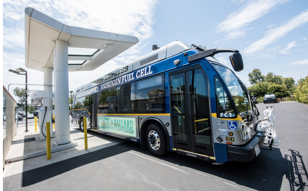
Figure 30. Fuel cell electric bus fueling at a hydrogen station (photo credit: NREL)
