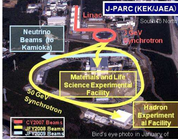
Figure 2.13: Bird's eye view of the J-PARC laboratory showing the primary components of its accelerator programs. To generate the high intensity neutrino beam, first the linear accelerator (Linac, red) accelerates protons into the 3 GeV Synchrotron (also red) called the rapid-cycle synchrotron (RCS). The RCS then injects some of its protons into the 50 GeV Synchrotron (yellow) called the main ring (MR), which currently runs at 30 GeV. Finally the MR protons are directed into a target material along the neutrino beamline (teal) [24].
