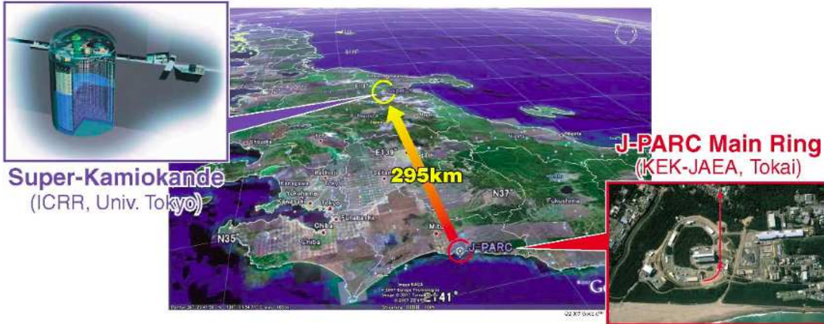
Figure 2.11: Birds eye view of the T2K experiment on the Japanese archipelago. An intense beam of neutrinos is produced at the J-PARC site (bottom right red box) using high energy protons. The beam is directed towards the Super-Kamiokande detector (top left blue box) at a distance of 295 km away from J-PARC.
