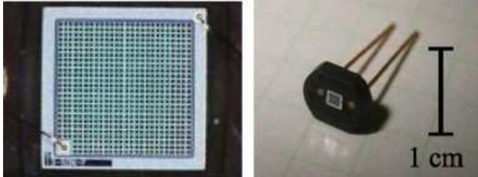
Figure 2.19: Photographs of the specially designed MPPC in T2K. A magnified face view is shown on the left with an entire unit shown on the right. Each device has 667-pixel sensors with an effective area of 1.3 \text{ mm} \times 1.3 \text{ mm} [19].
