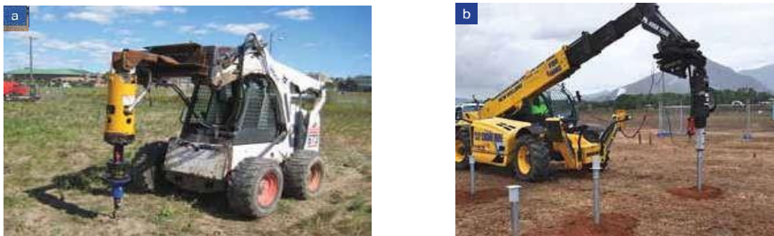
Figure 1.9 Typical Machines. (a) Backhoe; (b) Extend-boom. Lutenegeger (2011)
