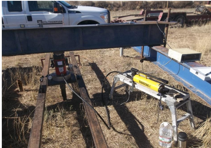
Figure 3.1 Compression set up (Courtesy of CTL|Thompson)
