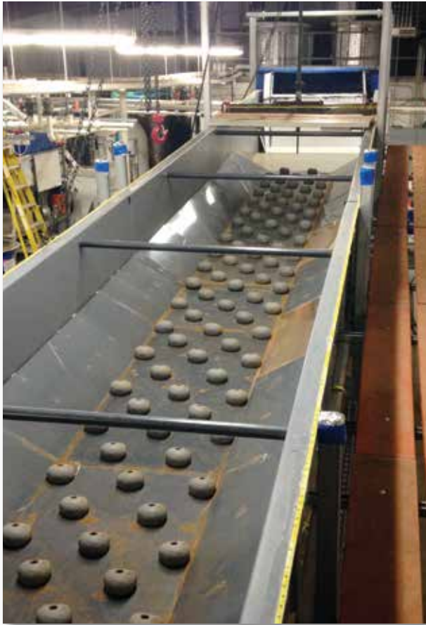
The CSU FPEL experimental rock ramp fishway, which was built to better understand the needs of small-bodied fishes as they attempt to traverse fish passage structures. The CSU FPEL plans to use the results of the experimental fishway in future recommendations to improve other field designs. Photo by Tyler Swarr.
