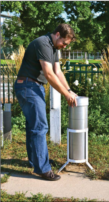
Figure 2. Jason Huitt, a weather observer at the CSU Weather Station, checks CSU's National Weather Service eight inch standard rain gage used at hundreds of Cooperative sites across the country for measuring precipitation. Photo by Kim Hudson
