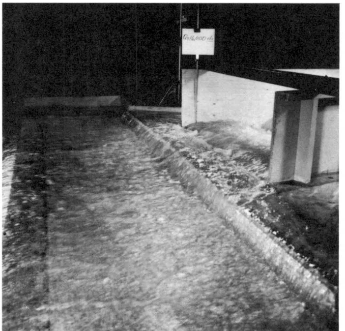
Figure 49. A view of the flow beyond the tertiary basin. Q = 16,000 cfs.
