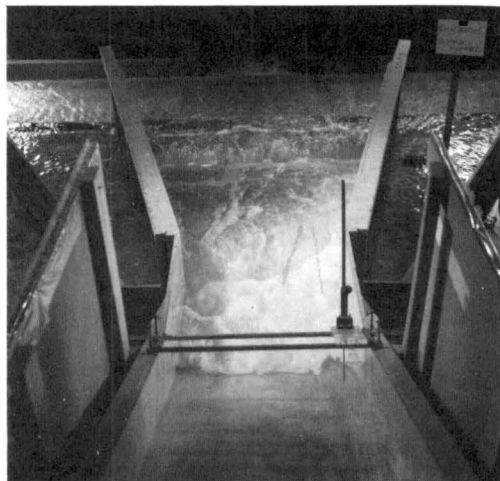
Fig. 6. View looking downstream from end of sloping sidewall. (Note the concentration of flow along right side of chute.)
