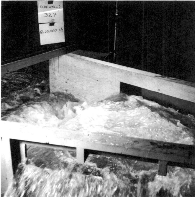
Figure 58. Q = 25,000 cfs. Primary and secondary basins. Note flow over the walls.
