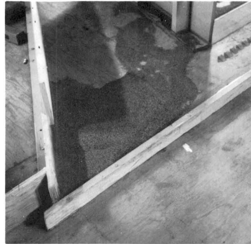
Fig. 14. Deposition pattern at lower end of side channel basin for Q = 25,000 cfs.
