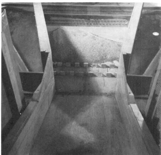
Fig. 9. Downstream view of sediment deposit after 20 minutes of model run time with a prototype discharge of 12,500 cfs. (Note the scour along the right side.)
