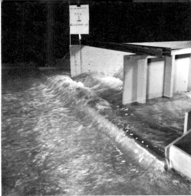
Figure 54. Q = 25,000 cfs. The flow spreads across the tertiary sill towards the river.
