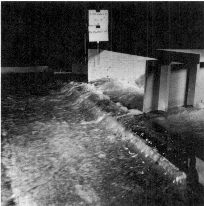
Figure 59. Q = 25,000 cfs. Flow beyond the tertiary sill. Note spread of flow.
