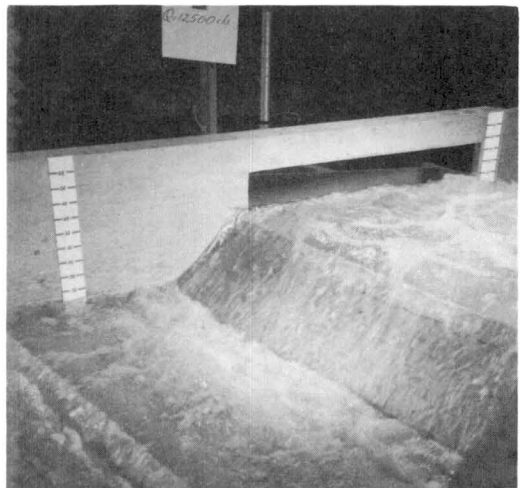
Plate 1. Comparable views of the operation of the energy dissipator for discharges of 6,000, 12,500, 19,000, and 25,000 cubic feet per second.
