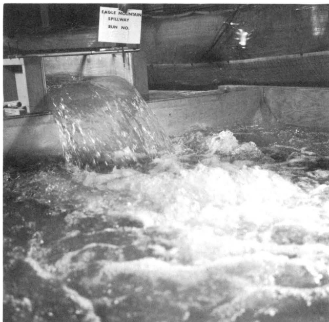
Fig. 33. Operation of circular energy dissipator
