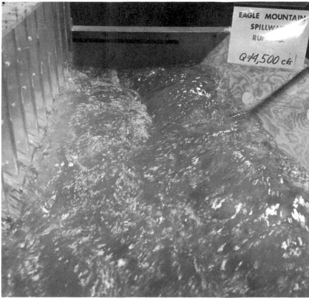
Fig. 19. Flow in side channel at a discharge of 14,500 cfs
