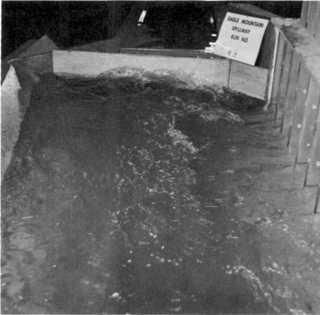
Fig. 26. Flow approaching transition section at a discharge of 22,300 cfs.
