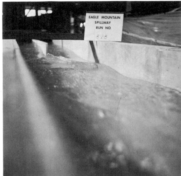
Fig. 31. Wave formation in conveyance channel
