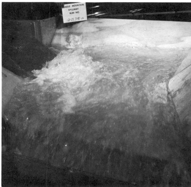
Fig. 35. Flow in energy dissipation basin at discharge of 21,340 cfs at design discharge
