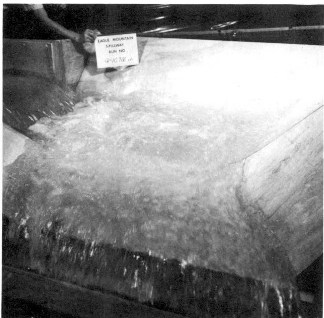
Fig. 34. Flow in energy dissipation basin at discharge of 10,700 cfs
