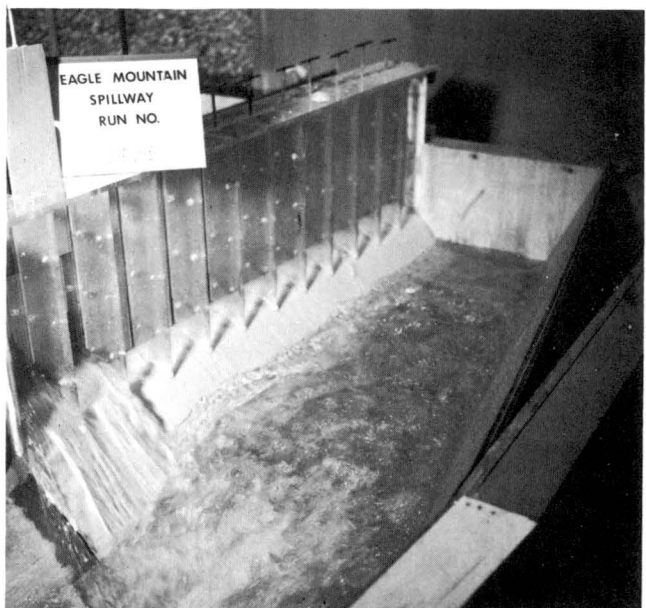
Fig. 22. Flow in side channel with gates 11 and 12 open
