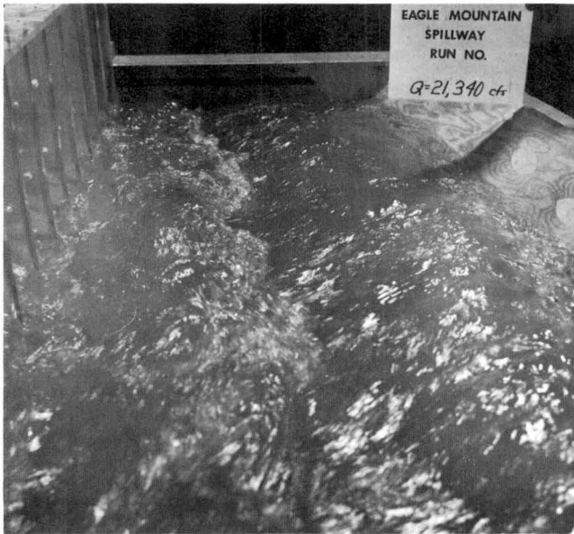
Fig. 15. Flow in side channel at design discharge
