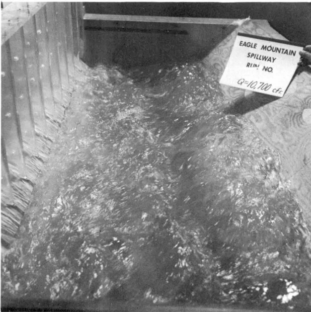
Fig. 20. Flow in side channel at a discharge of 10,700 cfs
