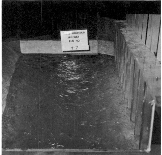
Fig. 28. Flow approaching transition section with one conduit closed at discharge of 8,400 cfs
