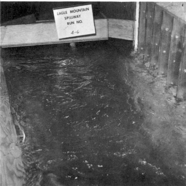
Fig. 27. Flow approaching transition section with one conduit closed at discharge of 7,380 cfs
