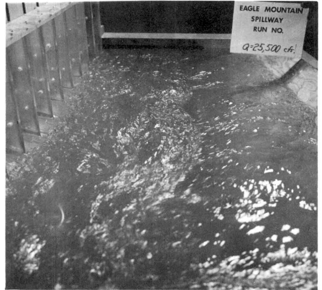
Fig. 17. Flow in side channel at a discharge of 25,500 cfs.
