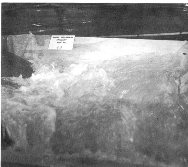
Fig. 36. Flow in energy dissipation basin at discharge of 27,000 cfs at design discharge
