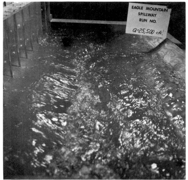
Fig. 18. Flow in side channel at a discharge of 25,500 cfs
