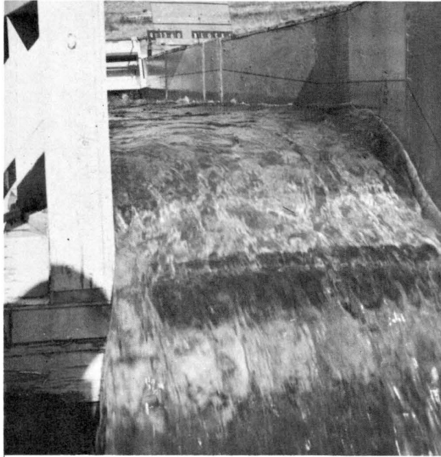
Figure 6(a) Water surface in Parshall flume - no modifications.
