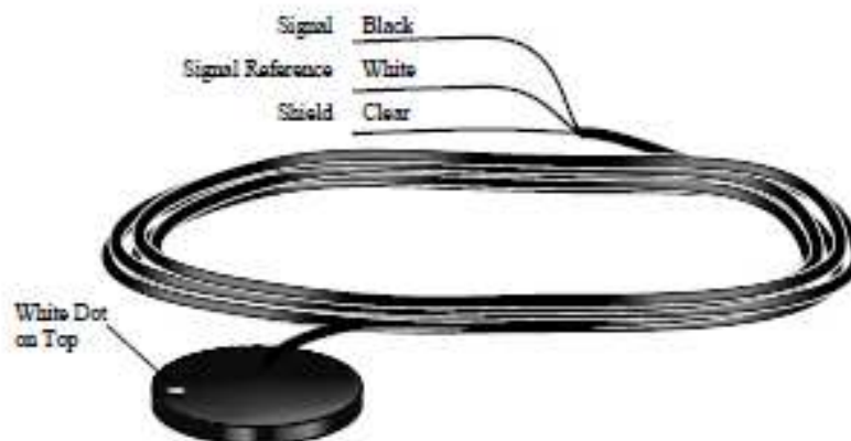
Figure 3.14: Soil heat flux plate installed on the fields on both underneath corn row and on the inter-row (Campbell Scientific, 2003).
