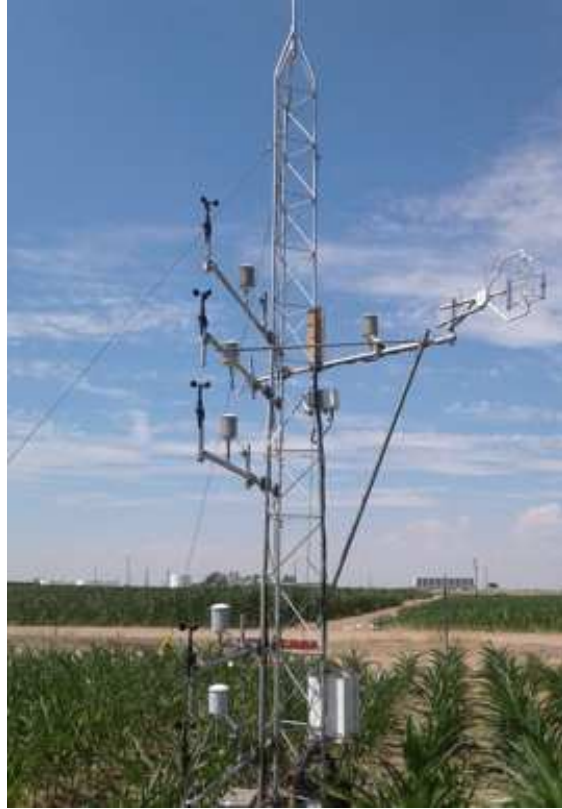
Figure 3.15: Aerodynamic flux tower with the eddy covariance system in 2017 on the field 2.
