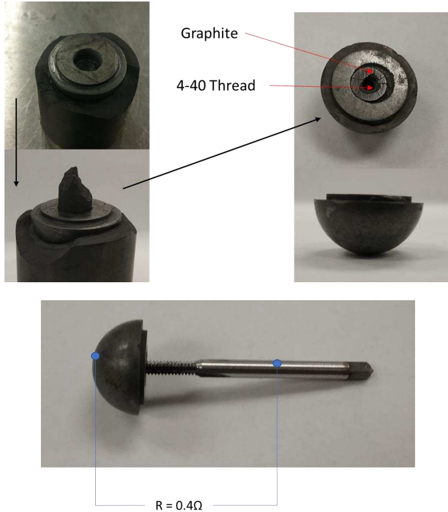
Figure 5.3: Schematic of procedure to add graphite mounting piece to hemispheres
