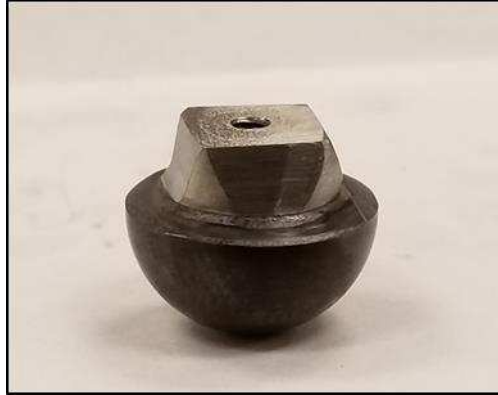
Figure 5.2: Hemisphere with Ti mounting piece attached
