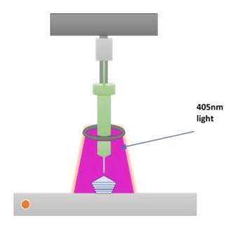
Figure 15. Schematic of the 3D printing process.
