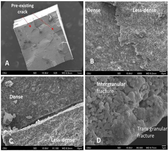
Figure 38. Fracture surface sintered HAp. (A) 25x magnification: evidence of pre-existing cracks. (B) and (C) 950x and 1100x magnification show two types of densification. (D) 6000x magnification: intergranular fracture in less-dense zones and trans granular fracture in denser zones of the sample.
