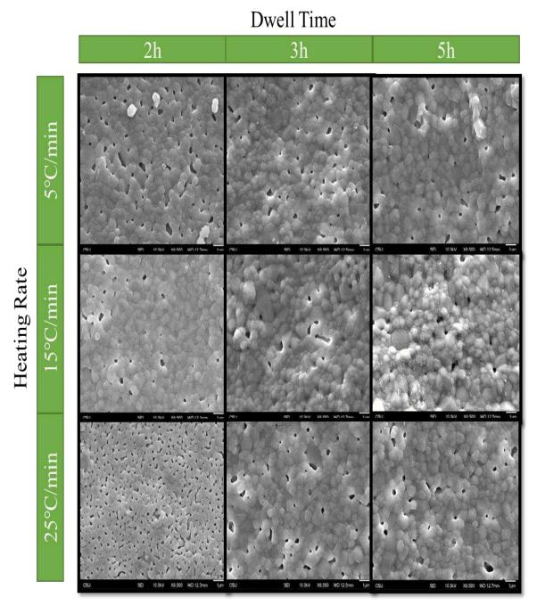
Figure 31. SEM images of surface densification of HAp samples resultant from the sintering DOE experiment.
