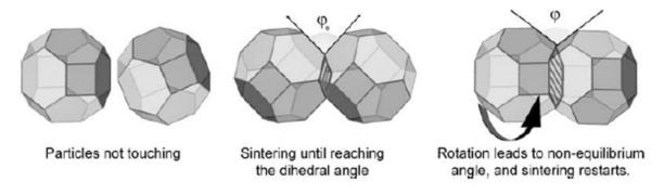
Figure 2.9. Evolution of dihedral angle in the sintering process [43]
