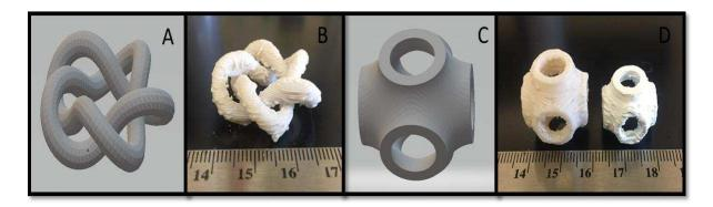
Figure 27. 3D printed complex structures. (B) and (D) are HAp complex structures produced from STL files (A) and (C), respectively. (D) contains a green body on the left and a sintered body on the right.
