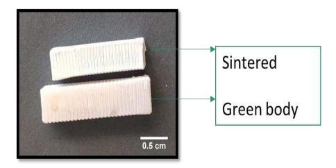
Figure 34. Shrinkage of HAp samples. The top sample corresponds to a sintered structure that had the same dimensions as the bottom sample (HAp/PEGDMA green body) before sintering.
