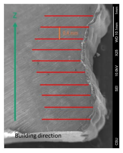
Figure 29. Layer cohesion of HAp samples. Red lines represent the location where layer division should be located, and the green arrow shows the building direction of HAp sample in the 3D printing process. The imaged face was polished, as described in Appendix 3.
