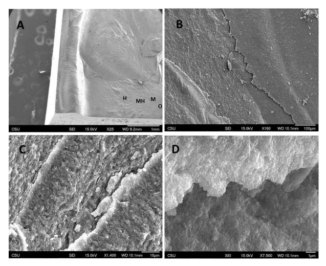
Figure 37. Fracture surface of green bodies. (A) 25x magnification: fracture origin can be seen O: origin, M: mirror fracture, MH: mist hackle, H: hackle. (B)150x magnification: fracture produced by the mirror pattern. (C) 1400x magnification: fracture from mirror pattern closer view (D) brittle fracture.
