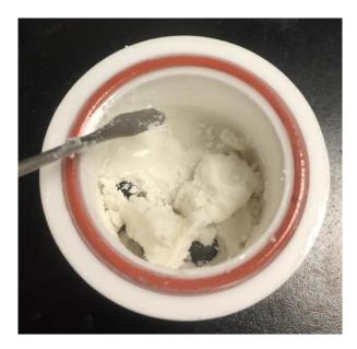
Figure 22. Dried HAp resin in milling jar with black agate milling balls.
