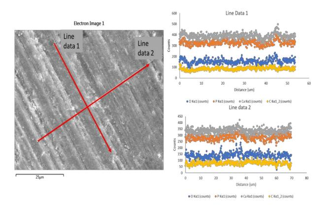
Figure 26. SEM image of HAp/PEGDMA green body surface. Red lines represent line scan of elemental composition done by EDS. Line data 1 and line data 2 show no significant change in element signal through the line scan length.
