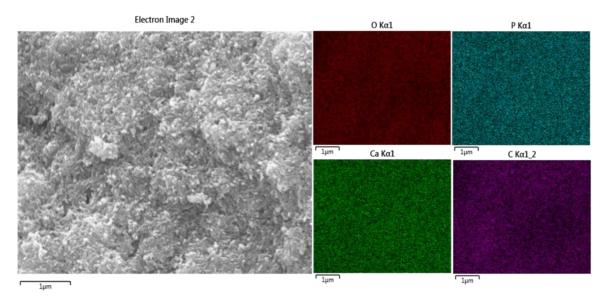
Figure 25. SEM image of HAp/PEGDMA green body surface. Lines are the product of the polishing process. Elemental maps of phosphorus, calcium, carbon, and oxygen are presented in green, blue, purple, and red, respectively.
