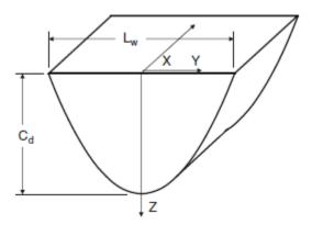
Figure 2.5. Cure depth profile of photopolymerization [23]
