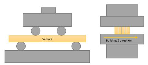
Figure 18. (A) Front view of flexural 4-point bending tester. (B) Lateral view of flexural 4-point bending tester. Testing direction for the samples was perpendicular to the building direction.
