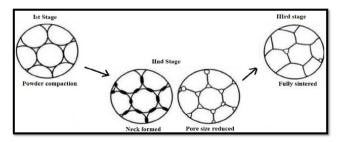
Figure 2.10. Stages of sintering [44].
