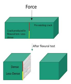
Figure 39. Schematic explaining cause for different densification. Red line represents preexisting crack and yellow line represents crack created after the flexural test.
