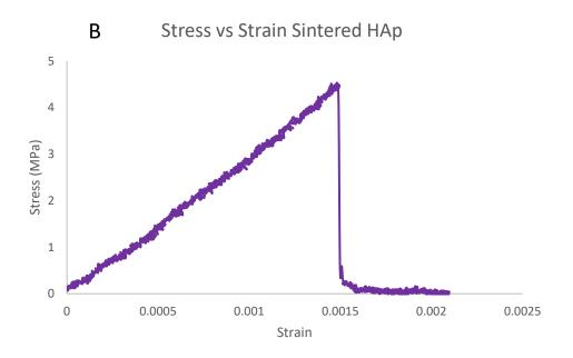
Figure 35. Characteristic flexural Stress vs. Strain curves obtained in 4-point bending for (A) HAp/PEGDMA green bodies and (B) HAp sintered structures.
