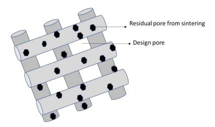
Figure 41. Sintered scaffold with residual and design porosity
