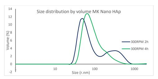
Figure 21. Particle size MK Nano HAp after ball milling treatment milled at the same speed and ball-to-powder ratio. Green line represents sample ball milled for 2h, and dark blue represents sample ball milled for 4h.
