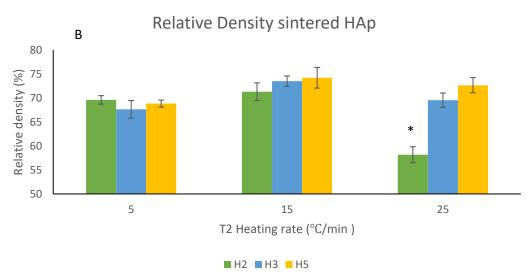
Figure 32. (A) Average grain size and (B) Relative density results of DOE of sintered structures. The asterisk represents a significant difference from the group at (p < 0.05)
