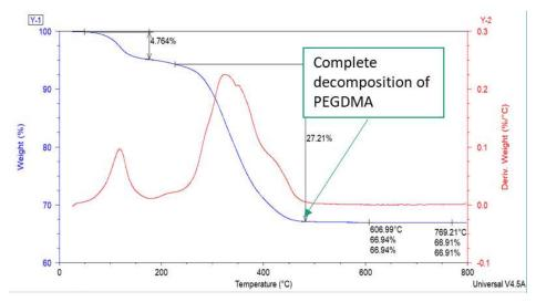
Figure 17. (A) SEM image of HAp densified surface using a heating rate (T1) faster than 5°C/min. Red circles show defects created by rapid degassing of burned PEGDMA. (B) Thermograph of HAp green body shows where total decomposition is reached ~450°C.
