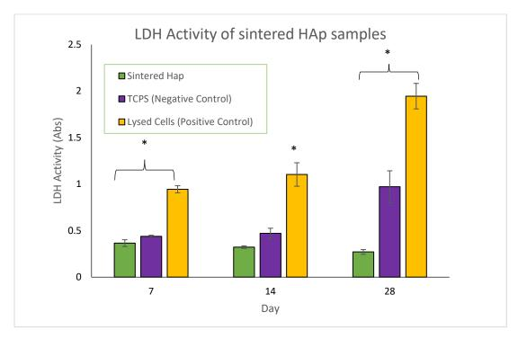
Figure 40. LDH Activity of sintered HAp samples for day 7,14 and 28.
