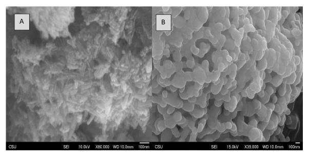
Figure 19.(A) As received Macron HAp particles. (B) Macron HAp after thermal treatment.
