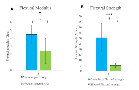
Figure 36. Flexural Modulus and flexural strength of HAp/PEGDMA and sintered HAp structures
