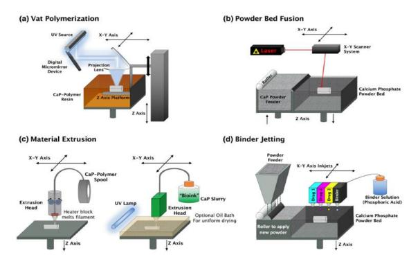
Figure 2.8. 3D printing technologies used in tissue engineering (a) vat polymerization, (b) powder bed fusion (c) material extrusion and (d) binder jetting [29]
