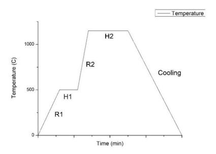
Figure 16. Sintering profile used to densify HAp structures. R1 and R2 are heating rates, and H1 and H2 are holding times
