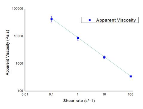
Figure 23. Shear thinning rheological behavior of HAp slurries.
