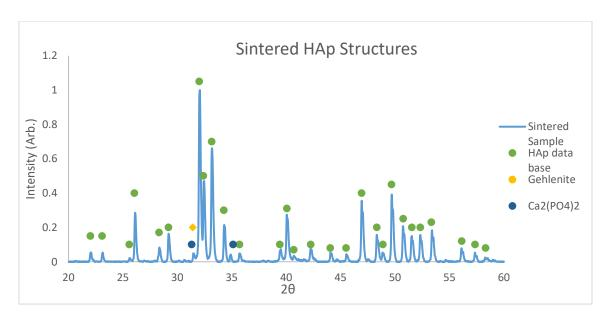
Figure 30. X-ray diffraction pattern of HAp sintered structures. Light blue is the data collected from the sample. Green, yellow and dark green are XRD data from the database of HAp, gehlenite and  $\beta$ -TCP, respectively.
