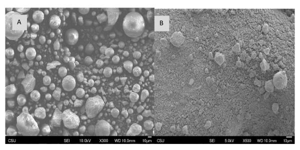
Figure 20. (A) As received MK Nano HAp particles (B) MK Nano HAp particles after ball milling treatment for 2h.
