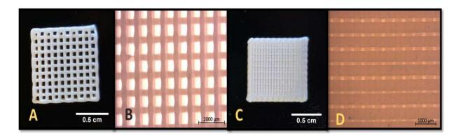
Figure 28. HAp/PEGDMA scaffolds (A) and (B) have ~600µm pore size, (C) and (D) have ~130µm pore size
