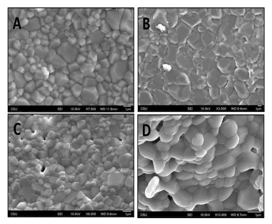
Figure 33 Different densification presented in HAp sintered structures. (A) top surface; (B) bottom surface; (C)lateral surface and (D) interior of HAp sintered structure.
