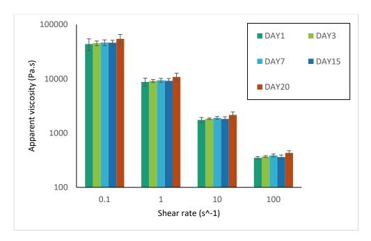
Figure 24. Viscosity of HAp slurries during the first 20 days after synthesis.
