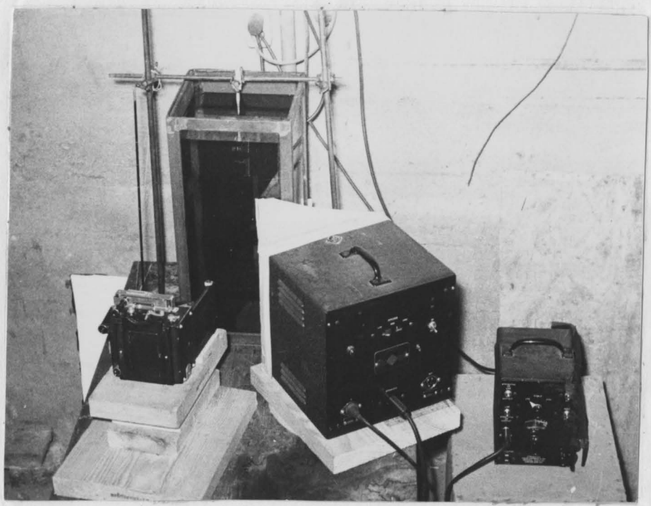
Fig. 1 -- Equipment for photographing falling particles.
