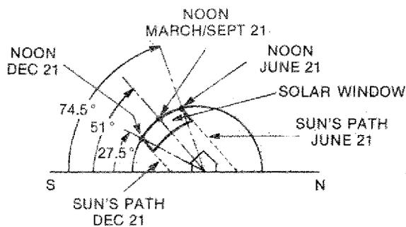
Figure 4: Cross-section of the solar window showing the angle of the sun at noon for 39°N latitude.
