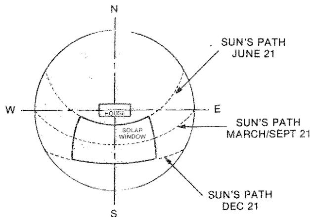
Figure 3: Plan view of the solar window.
