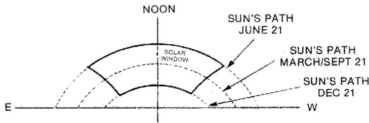
Figure 2: South-facing view of the solar window.
