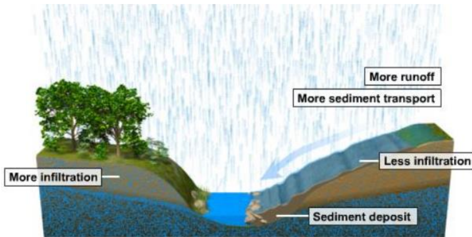
Figure 5-1: Influences of ground cover loss on runoff, groundwater, and sediment transport (University Corporation for Atmospheric Research, 2010).
