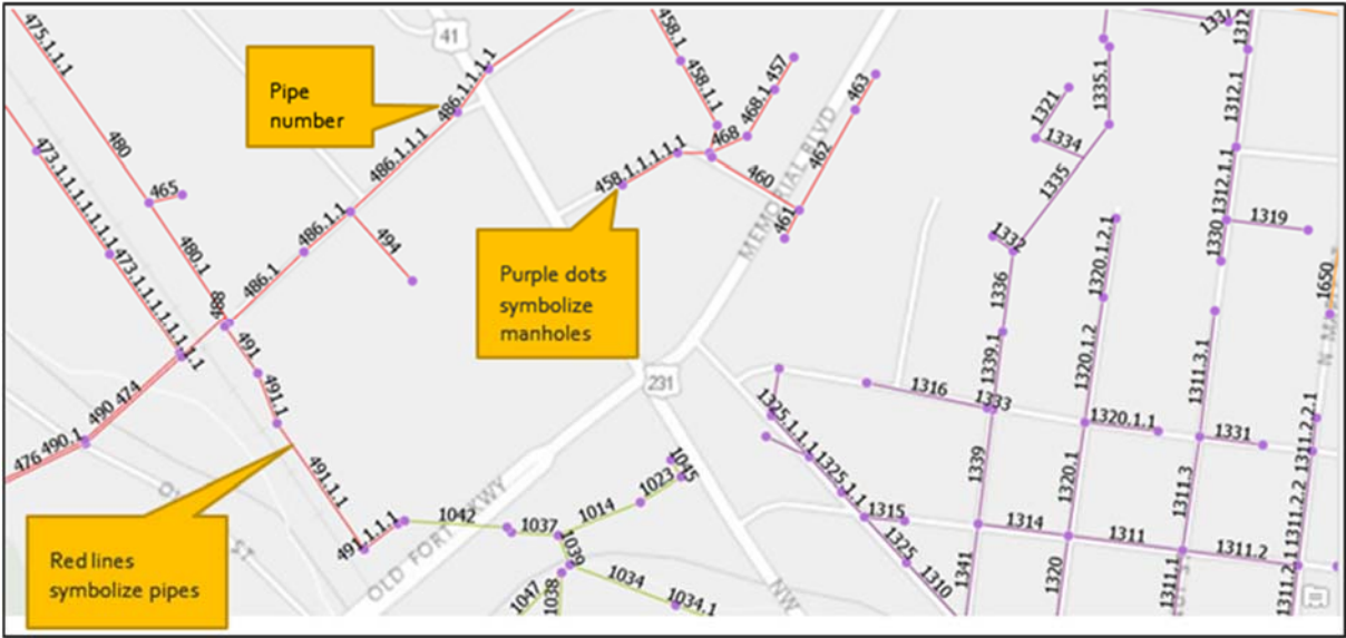
Figure 4-20: An example of the manholes and pipes at City A imported from the GIS system.
