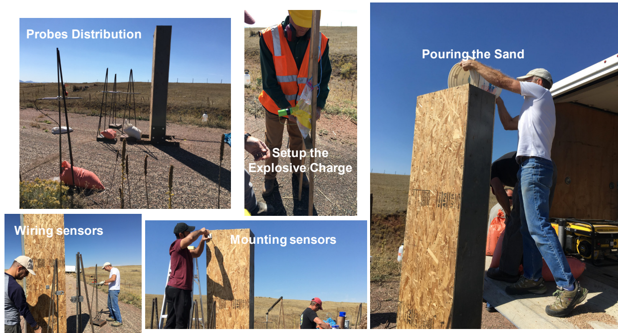
Figure 5.55 W SaW blast wall test setup.
