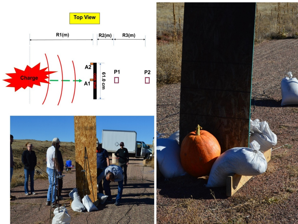
Figure 5.28 OSB wall blast test setup.
