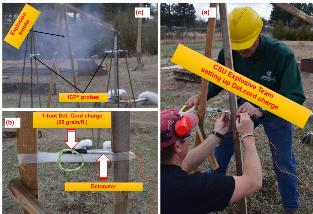
Figure 5.12 a. Setting up the charge, b. Detonating cord charge test-I setting c. charge detonation.
