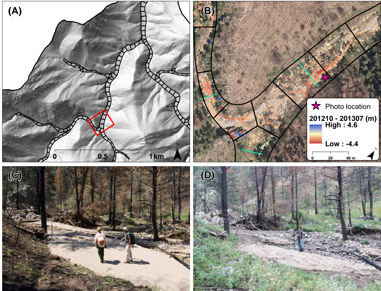
Figure 4.12: Illustration of channel incision and widening in Skin Gulch during T1 as a result of summer thunderstorms followed by snowmelt. The red square in (A) shows the location of the valley bottom segments in (B), and the red star in (B) shows the location of the photos in (C) and (D). Green lines in (B) represent surveyed cross sections, and contour intervals are 1 m (thin lines) and 5 m (thick lines). The photo in (C) was taken on 11 August 2012 and shows the extensive deposition that occurred in the first two months after the fire. (D) shows the same location after spring snowmelt. Maximum erosion was ~1.0 m near the photo location.
