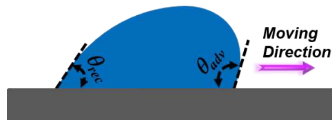
Figure 2: Schematic showing the advancing (forward) and receding (trailing) angles that develop as a droplet moves across a surface
