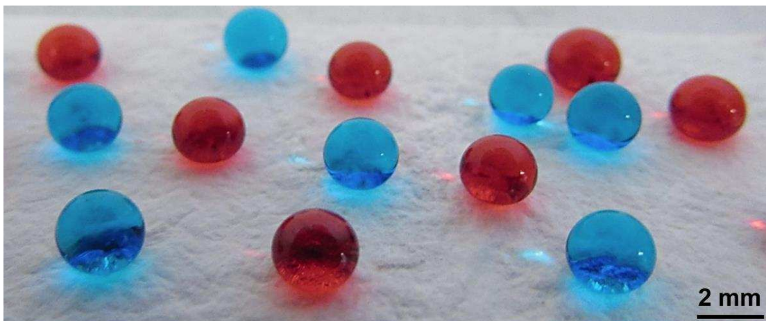
Figure 9: Super-repellency of both hexadecane (red; 27.1 \text{ mN m}^{-1} ) and water (blue, 72.1 \text{ mN m}^{-1} )
