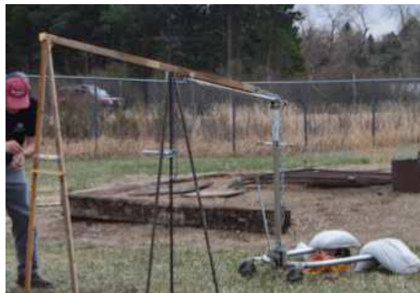
Figure 8: Picture of the stand used to support the explosive charge during tests.
