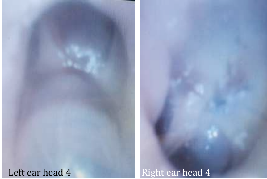
Figure G.2: Remaining two ears from September blast test. Based on visual analysis of the eardrum with the borescope, there were no signs of rupture or other damage.
