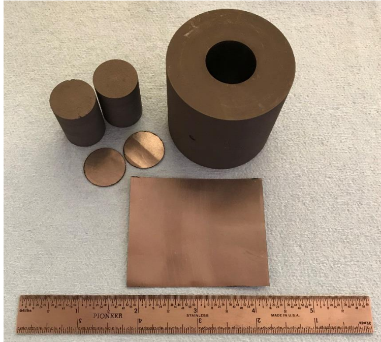
Figure 5.2. Graphite die (x1), graphite punches (x2), graphite discs (x2) and graphite liner (x1) used to sinter MSC specimens.
