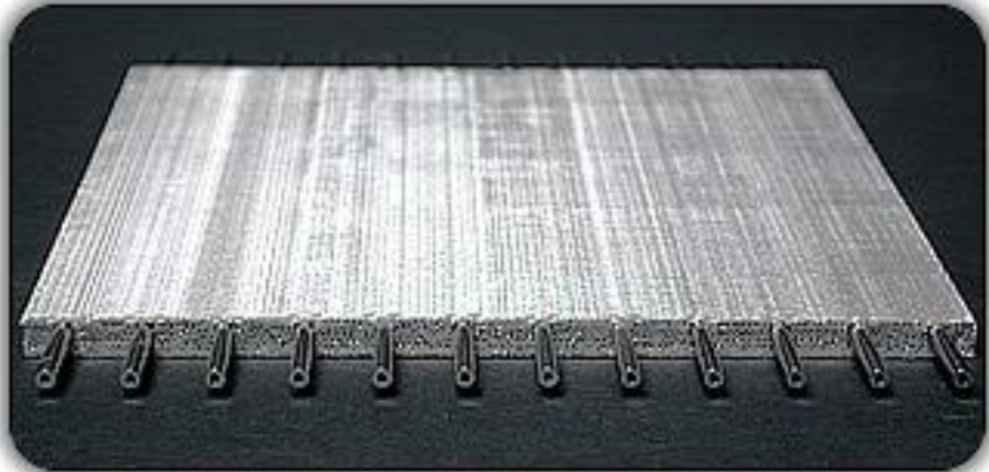
Figure 1.4. A metal open-cell foam demonstrating multifunctionality by functioning as both a catalyst support structure and as a heat exchanger. [55]
