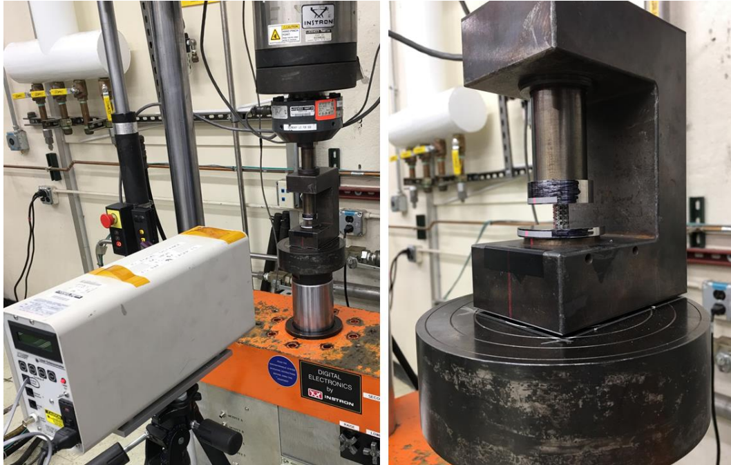
Figure 4.7. Mechanical compression test setup to characterize the NiTi open-cell foam specimens to failure. (LEFT): Overall test setup showing the Instron 1332 hydraulic load frame, non-contact laser extensometer, and custom-designed compression loading fixture. (RIGHT): Close-up of the compression loading fixture showing a foam specimen installed prior to test initiation, laser extensometer reflective targets, and hardened steel platens.
