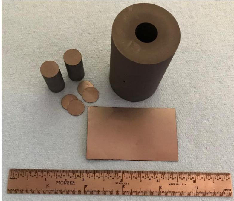
Figure 4.2. Graphite die (x1), graphite punches (x2), graphite discs (x4) and graphite liner (x1) used to sinter the NiTi open-cell foam specimens.
