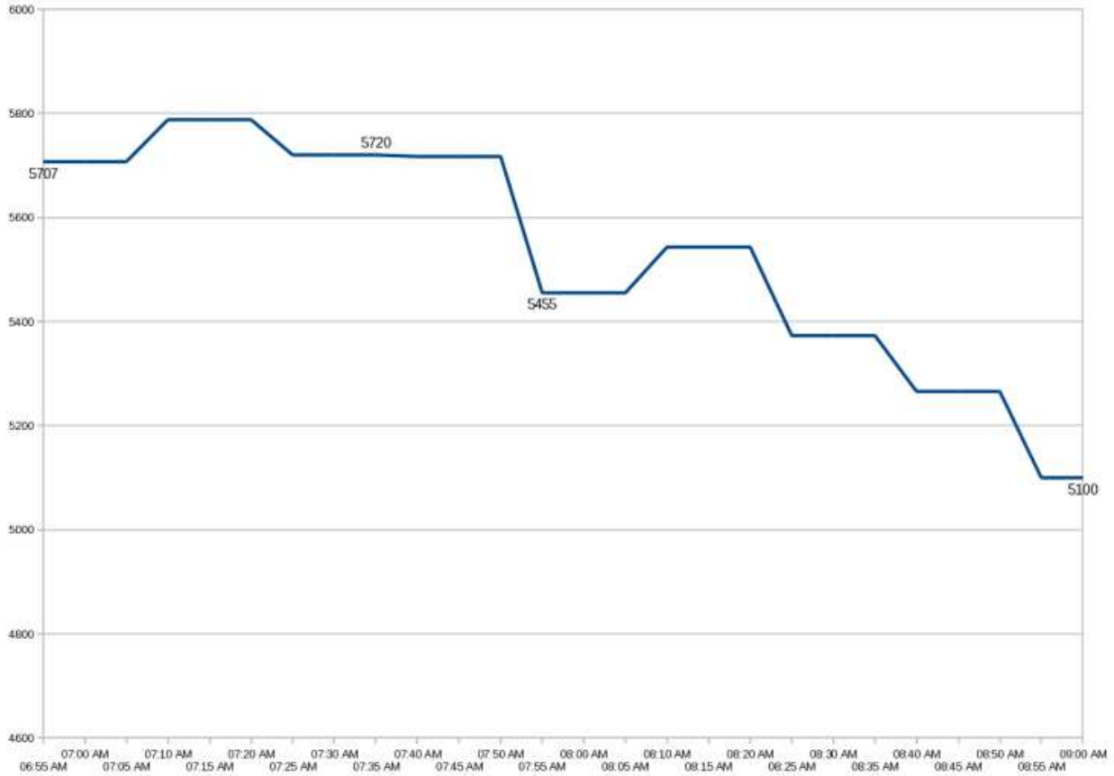
Figure 10 - Substation Load in kW
