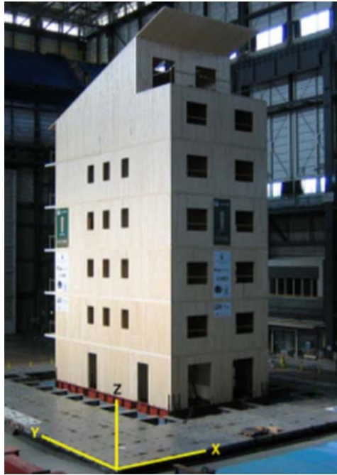
Figure 2.7: 7-story SOFIE structure, Ceccotti et al. (2013)
