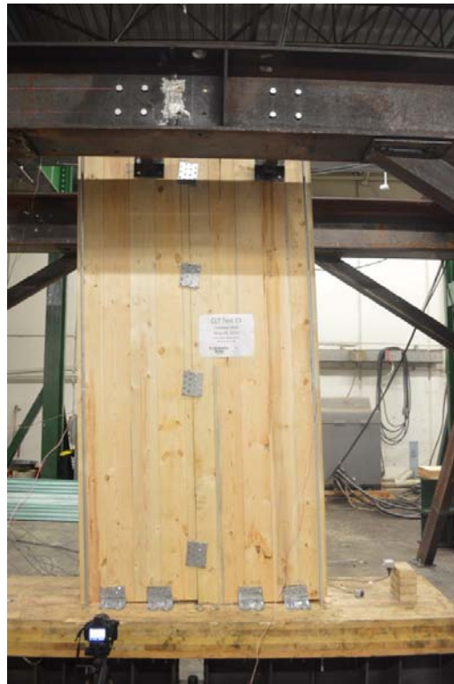
Figure 4.50: Test 23, shear wall with (2) 2ft panels with vertical joint
