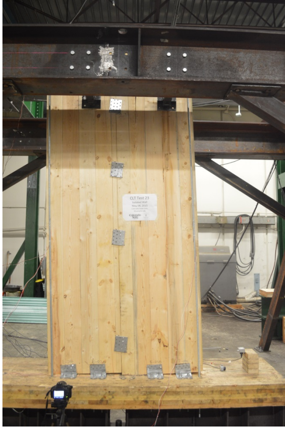
(a) multi-panel configuration rocking during the test
