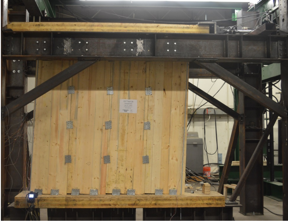
Figure 4.51: Test 26, shear wall with (4) 2ft panels with vertical joint
