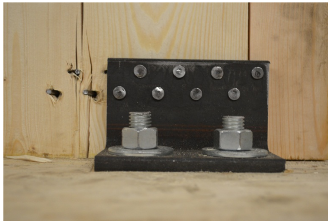
Figure 4.36: A1 type connector after test
