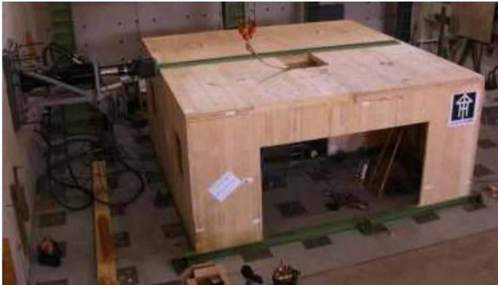
Figure 2.4: Specimen for psuedo-dynamic testing, third configuration Lauriola et al. (2006)
