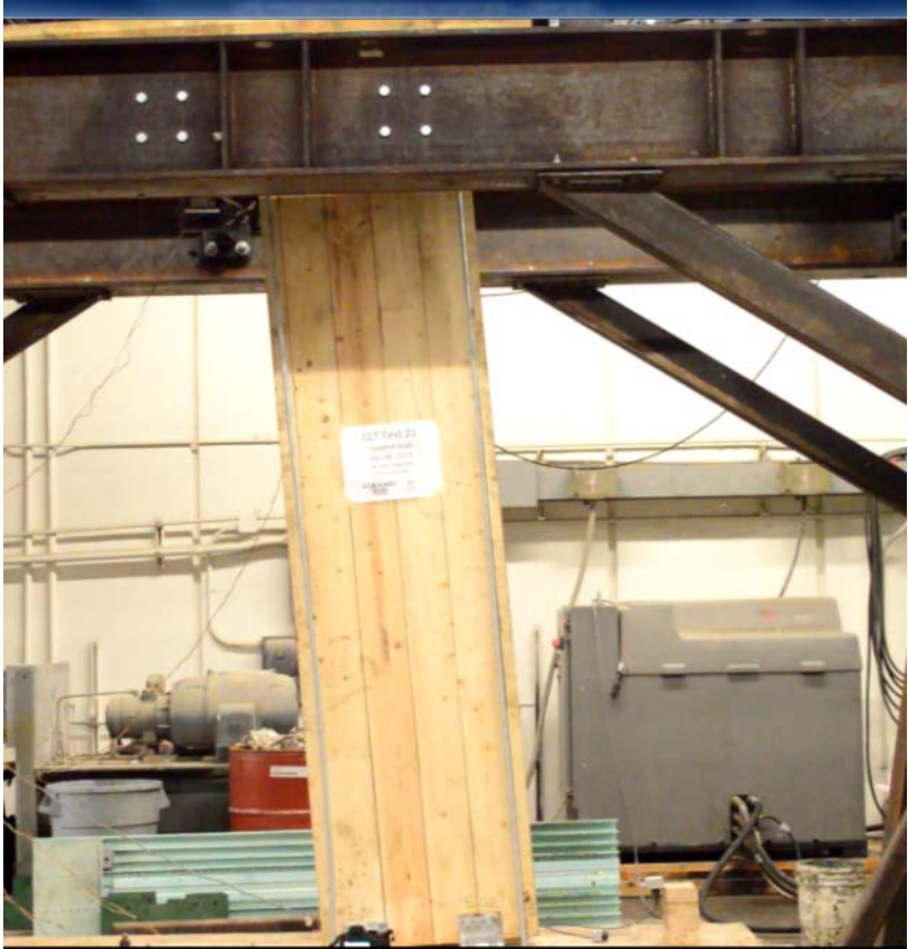
(a) CLT panel rocking during the test
