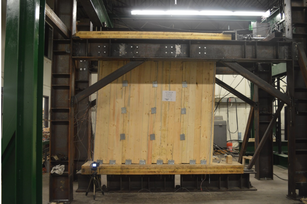
(a) multi-panel configuration rocking during the test
