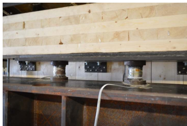
Figure 4.37: Floor diaphragm support
