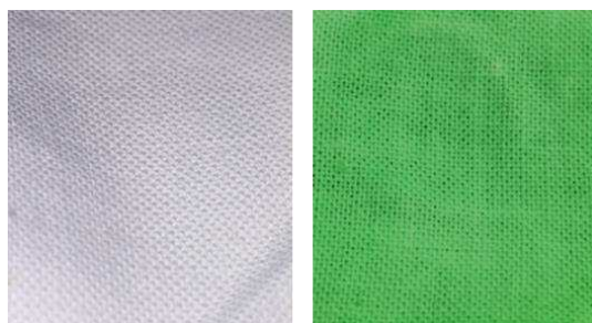
Figure 3.5. Images of natural cotton used (left) and the uniformly grown MOF on cotton material (right).
