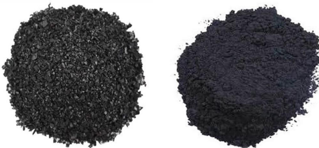
Figure 1.7: GAC ( left ) and PAC ( right ) (Calgon Carbon)
