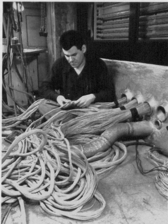
Lawrence Phelps assembles the wiring for a pipe organ.
