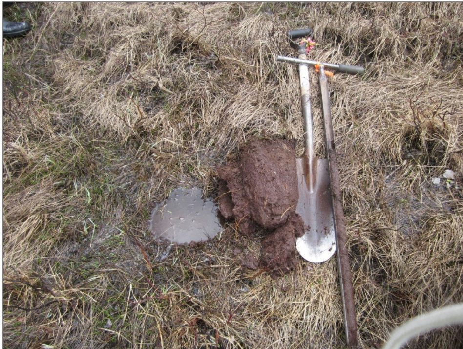
Figure 2. Soil cores taken with a sharpshooter shovel and a gouge auger.
