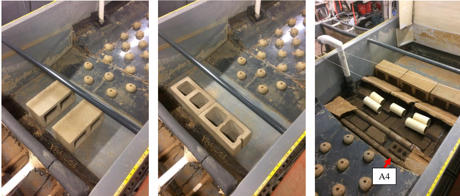
Figure 3-1. — Photographs of the orientations of the cinderblocks in the downstream refuge area for the Flathead Chub and Stonecat trials (left) and for the Arkansas Darter trials (center). Photo of the upstream refuge area with the uppermost PIT tag antenna (A4; right).
