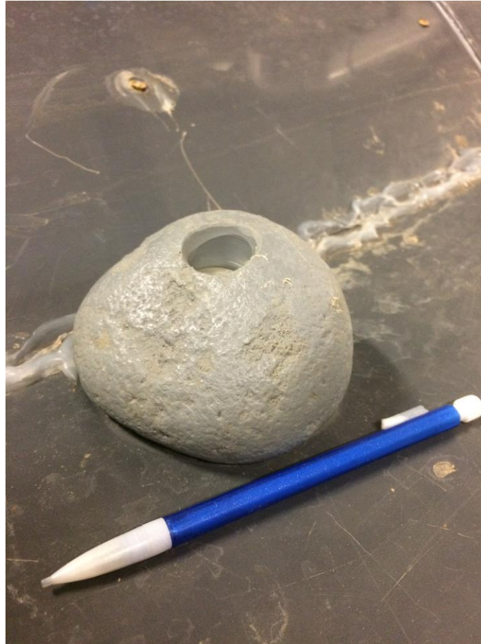
Figure 1-3. — Photograph showing the shape of the roughness elements used throughout the fishway. Roughness elements were identical molded polyethylene rocks and could be rearranged by bolting the roughness elements to the floor of the PVC fishway. The sloped side of the roughness elements were oriented upstream to mimic the orientation of cobbles in streams.
