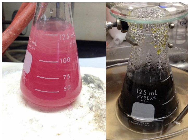
Figure S2.12. Photographs of reaction solution following the procedure used in the 2014 synthesis 2 prior to heating (left) and after heating at 80 °C for two hours (right).
