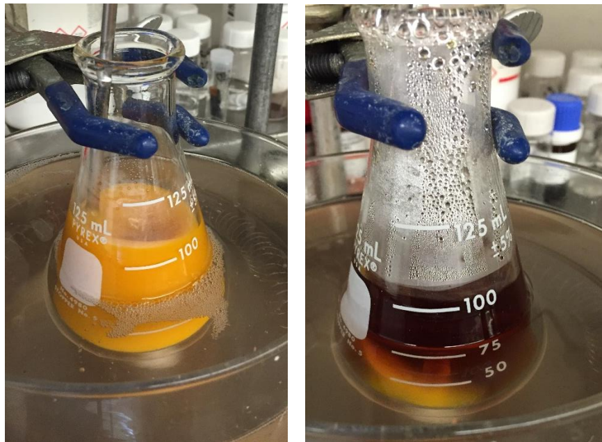
Figure S2.10. Photographs of reaction solution following the Original 1 synthesis procedure: V_2O_5 solution prior to addition of cobalt or tungstate (left) and after heating for 40 minutes at 70^\circ\text{C} for 40 minutes in the presence of cobalt and tungsten (right).
