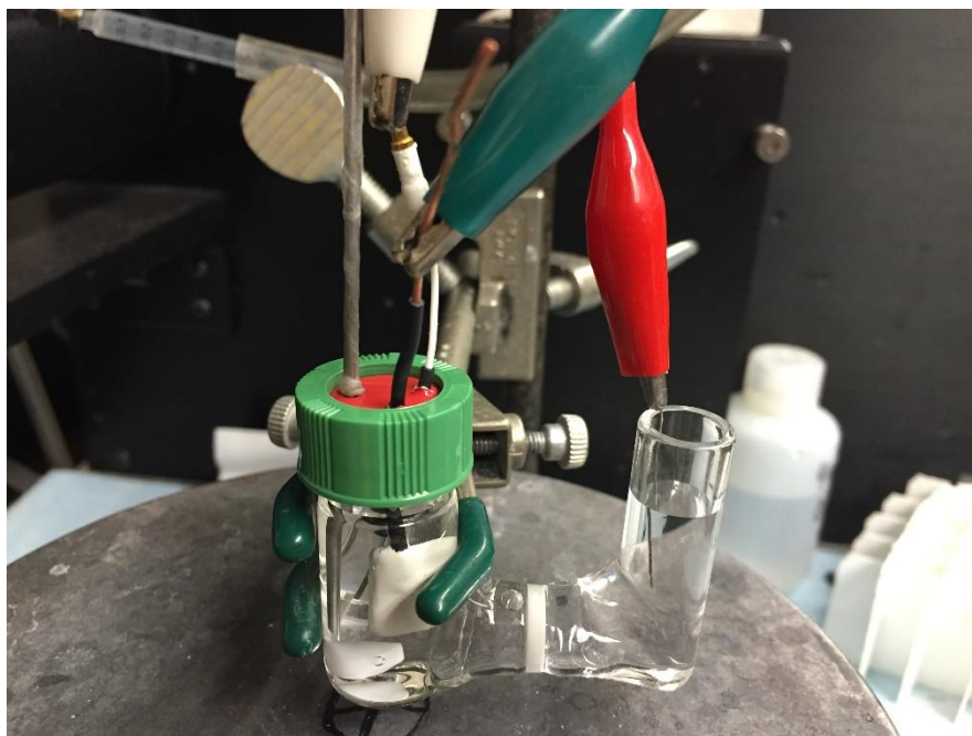
Figure S3.6. Photograph of the custom built U-cell employed for O 2 quantification experiments.
