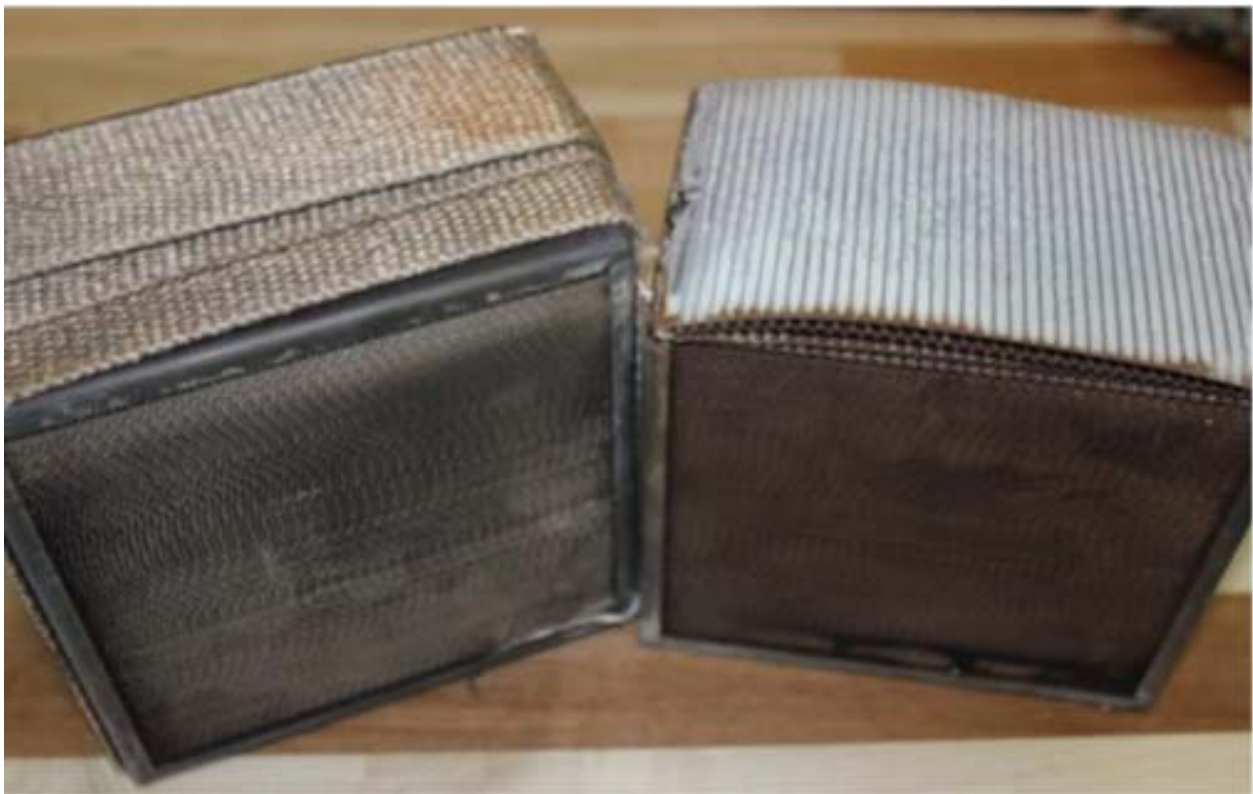
Figure 2.1: Catalyst modules. Intact module on left for performance testing and partially disassembled module on left for elemental analysis
