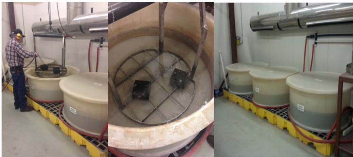
Figure 2.5: Collage of photos of the washing process. Left: Catalyst modules being blown with compressed air. Middle: Modules on a rack lowered into the acid bath. Right: the caustic soda, rinse water and acid baths
