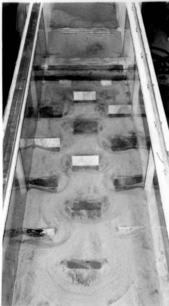
Fig. 22. Top Views with all Baffles 12" High and 2' Wide. Lateral Spacing 6' and Longitudinal Spacing 2' from Center to Center Q = 400 CFS
