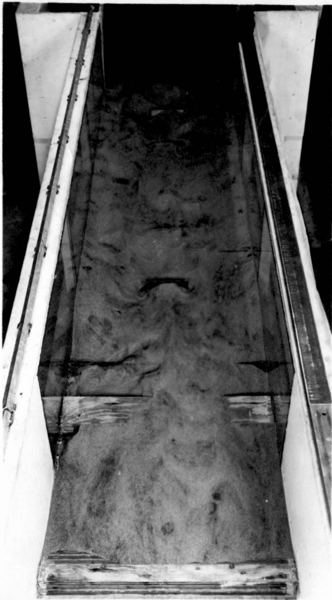
Fig. 14. Top Views with all Baffles 6" High and 2' Wide. Lateral Spacing 6' and Longitudinal Spacing 2' from Center to Center. Q = 250 CFS
