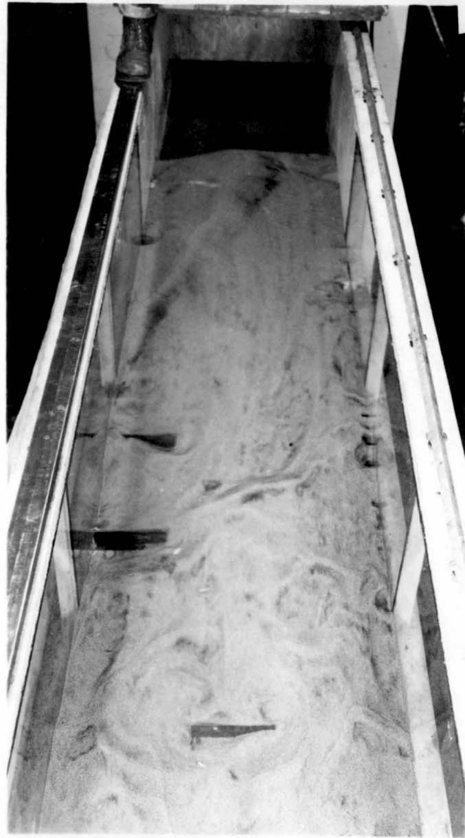
Fig. 16. Top Views with all Baffles 6" High and 2' Wide. Lateral Spacing 6' and Longitudinal Spacing 2' from Center to Center. Q = 400 CFS
