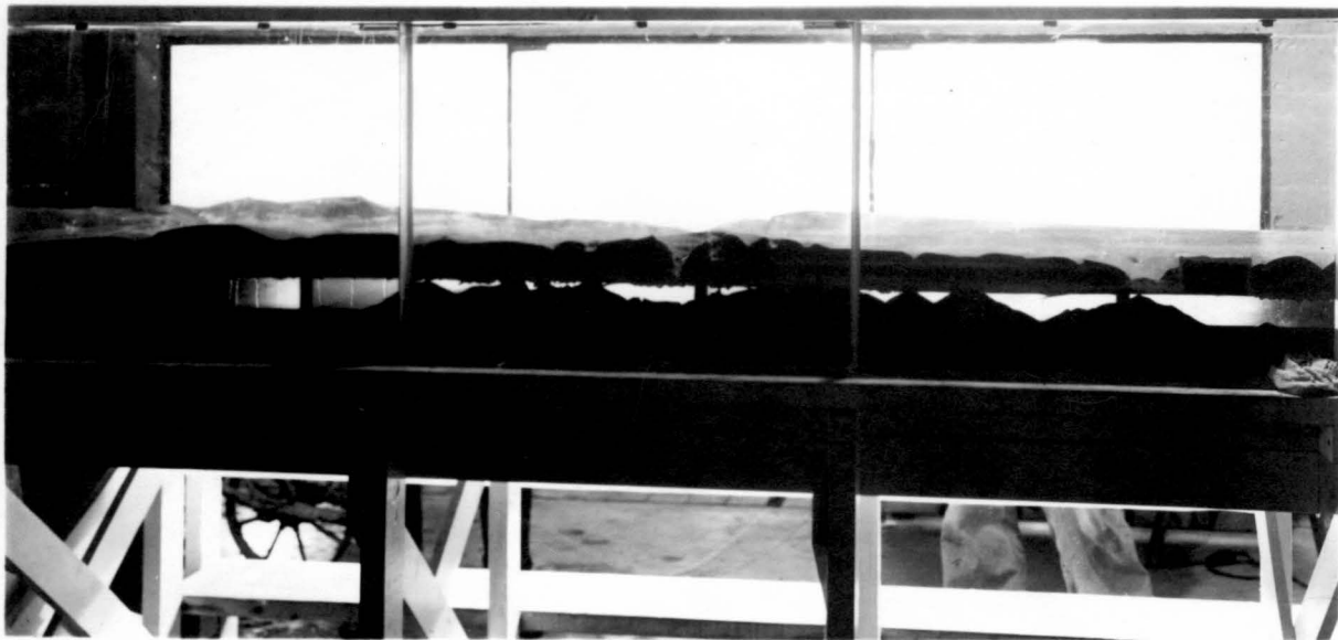
Fig. 15. Side Views with all Baffles 6" High and 2' Wide. Lateral Spacing 6' and Longitudinal Spacing 2' from Center to Center. Q = 400 CFS
