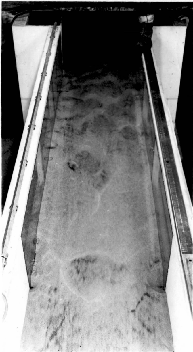
Fig. 18. Top Views with all Baffles 6" High and 2' Wide. Lateral Spacing 6' and Longitudinal Spacing 2' from Center to Center. Q = 800 CFS
