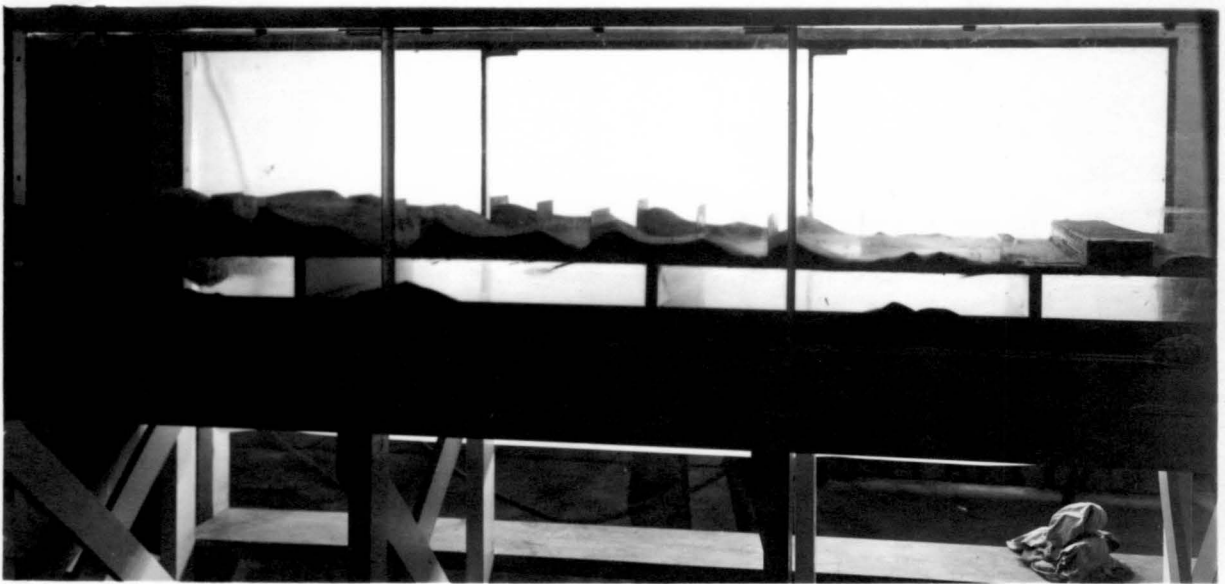
Fig. 19. Side Views with all Baffles 12" High and 2' Wide. Lateral Spacing 6' and Longitudinal Spacing 2' from Center to Center. Q = 250 CFS
