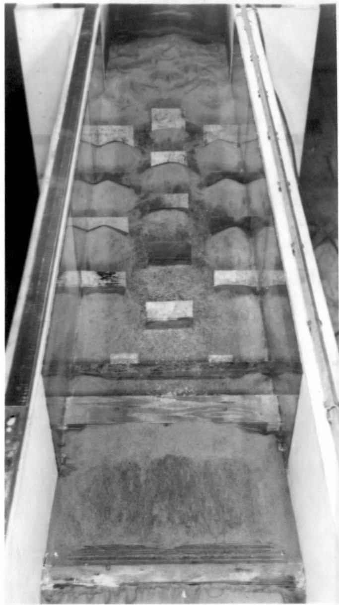
Fig. 28. Top Views with all Baffles 2' Wide. Two Upstream Rows 18" High and Remaining Rows 12" High. Lateral Spacing 6' and Longitudinal Spacing 2' from Center to Center. Q = 400 CFS
