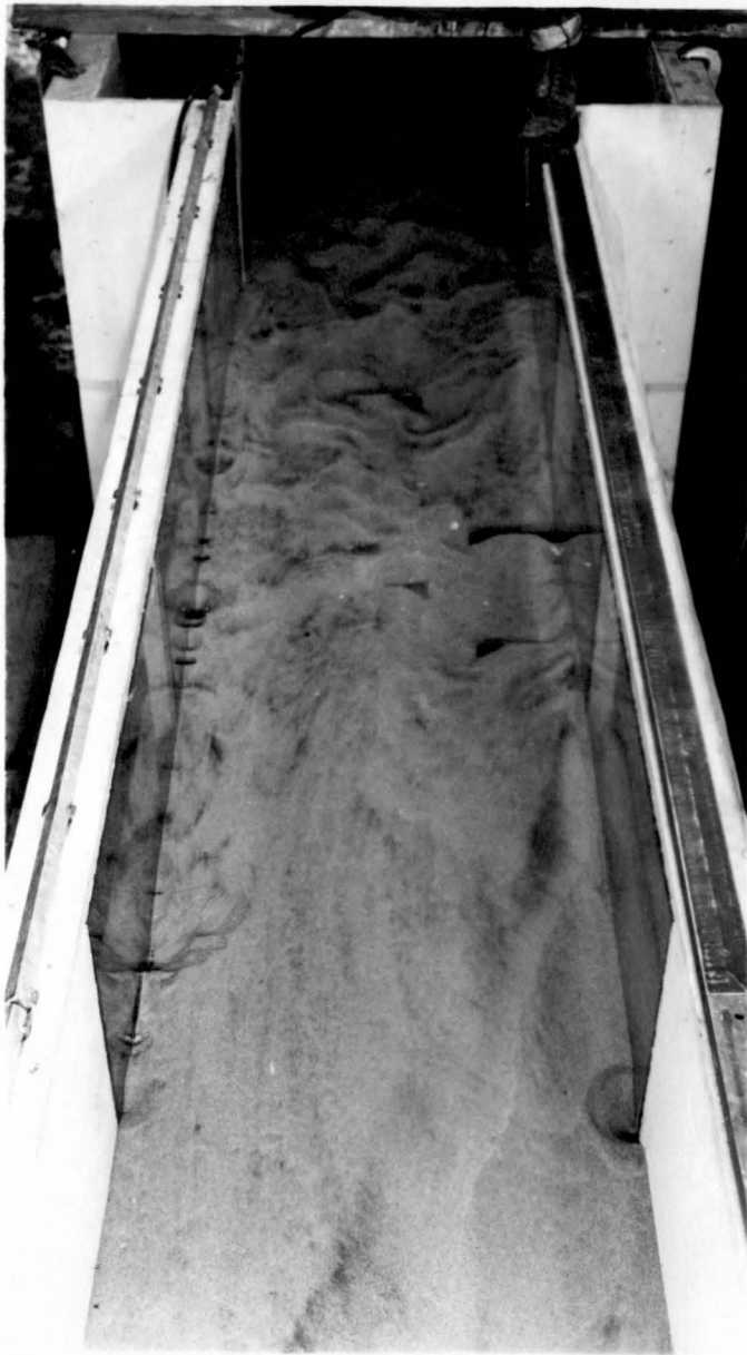
Fig. 16. Top Views with all Baffles 6" High and 2' Wide. Lateral Spacing 6' and Longitudinal Spacing 2' from Center to Center. Q = 400 CFS
