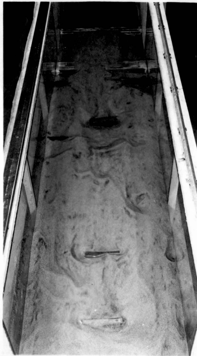
Fig. 14. Top Views with all Baffles 6" High and 2' Wide. Lateral Spacing 6' and Longitudinal Spacing 2' from Center to Center. Q = 250 CFS
