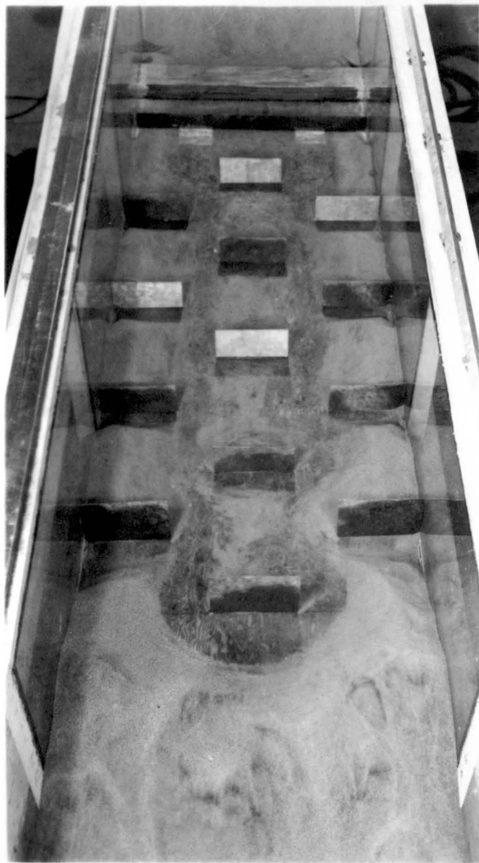
Fig. 26. Top Views with all Baffles 2' Wide. Two Upstream Rows 18" High and Remaining Rows 12" High. Lateral Spacing 6' and Longitudinal Spacing 2' from Center to Center. Q = 250 CFS
