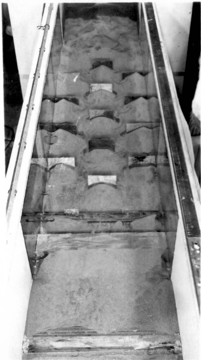
Fig. 22. Top Views with all Baffles 12" High and 2' Wide. Lateral Spacing 6' and Longitudinal Spacing 2' from Center to Center Q = 400 CFS
