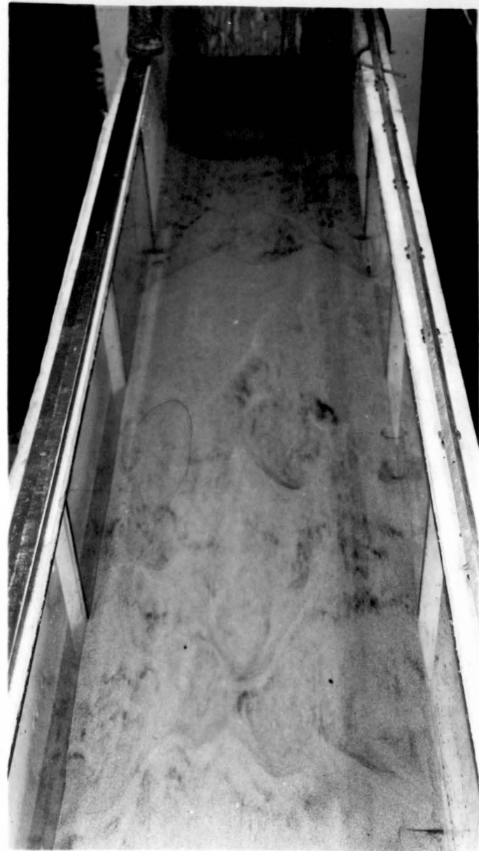
Fig. 18. Top Views with all Baffles 6" High and 2' Wide. Lateral Spacing 6' and Longitudinal Spacing 2' from Center to Center. Q = 800 CFS
