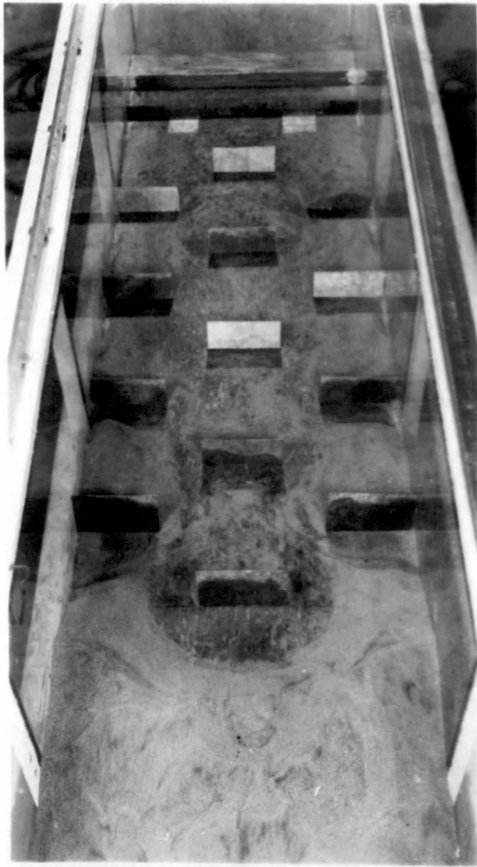
Fig. 28. Top Views with all Baffles 2' Wide. Two Upstream Rows 18" High and Remaining Rows 12" High. Lateral Spacing 6' and Longitudinal Spacing 2' from Center to Center. Q = 400 CFS
