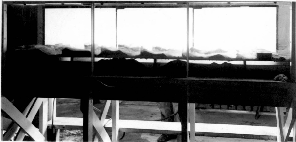
Fig. 23. Side Views with all Baffles 12" High and 2' Wide. Lateral Spacing 6' and Longitudinal Spacing 2' from Center to Center Q = 800 CFS
