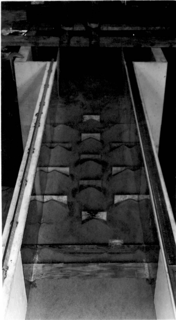
Fig. 20. Top Views with all Baffles 12" High and 2' Wide. Lateral Spacing 6' and Longitudinal Spacing 2' from Center to Center.
