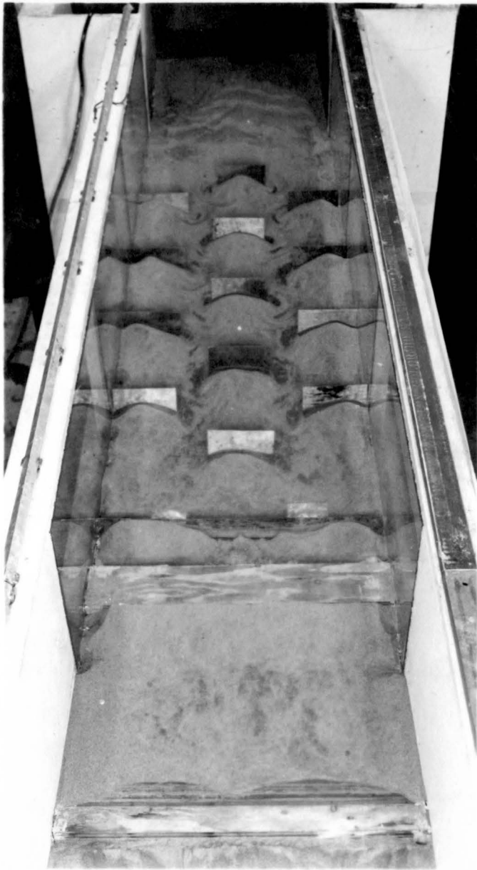
Fig. 24. Top Views with all Baffles 12" High and 2' Wide. Lateral Spacing 6' and Longitudinal Spacing 2' from Center to Center Q = 800 CFS
