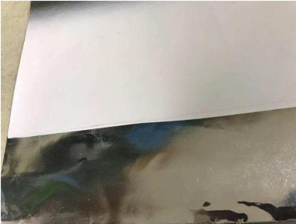
4. Use tweezers to pick up to pick up the nanofiber bundle and pull it away from the aluminum foil and onto the surrounding counter. Finish rolling up the nanofiber bundle.
