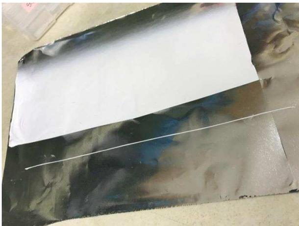
5. Repeat with remainder of the nanofiber sheet. If the final nanofiber bundle created with the last edge of the electrospun sheet is far too small in diameter (i.e. if it is similar in diameter to a strand of hair) then discard.
