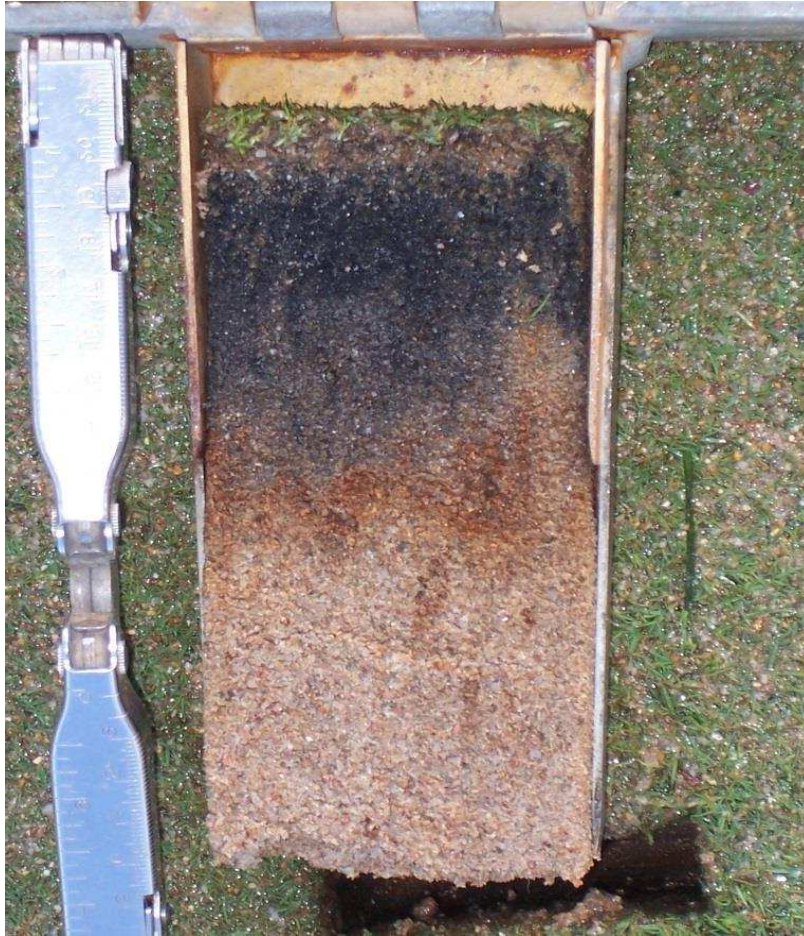
Photo 1.1. Black layer underneath putting green surface.
