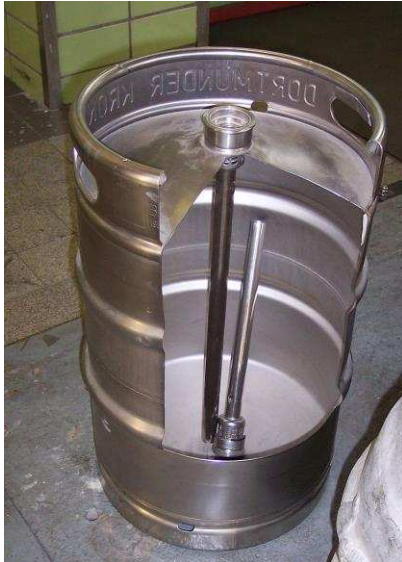
Figure 8.1. Cross-section of half barrel keg The downtube dispenser and spear valve in the center of the keg can be seen in a cross section. Image source ( https://es.wikipedia.org/wiki/Barril_de_cerveza )
