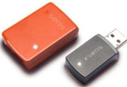
Figure 2.2. Xsens IMU sensor and antennae dongle (Xsens, 2015)
