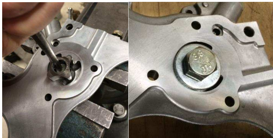
Figure 3-7. Removing oil pump drive shaft and pinion (left). Bolt used to plug oil pump shaft bore (right).
