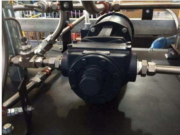
Figure 3-10. Internal gear pump used to pressurize cooling system.
