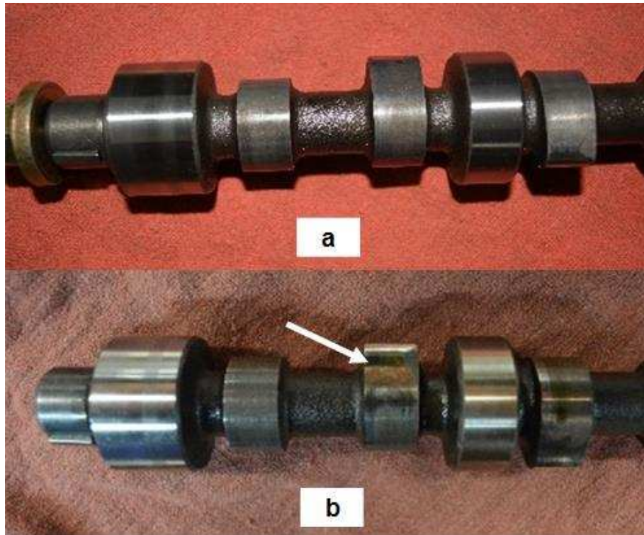
Figure 6-17. Photos of camshaft before (a) and after (b) testing with arrow indicating slight wear from insufficient lubrication at sliding contact between lobe and lifter.
