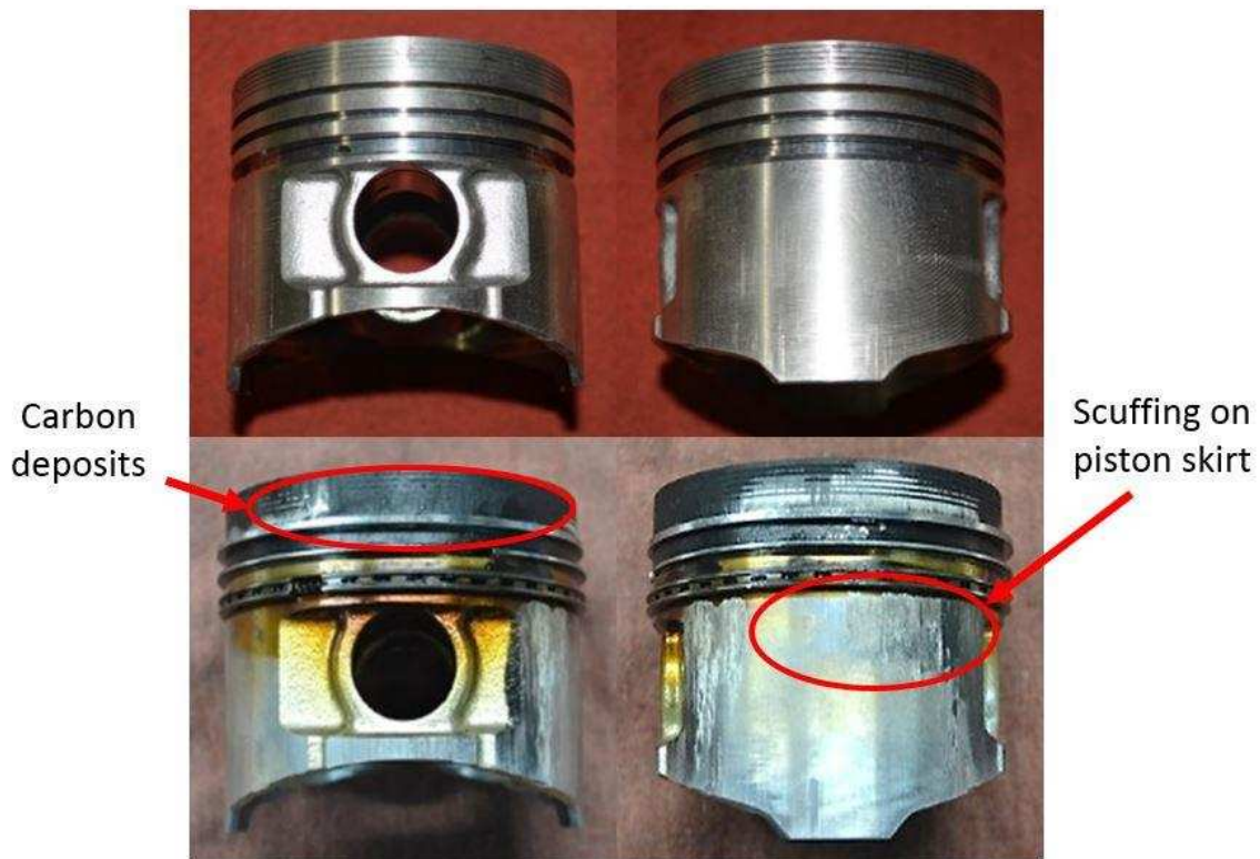
Figure 6-13. Documentation of piston condition showing piston from cylinder 1 before (top) and after (bottom) testing.
