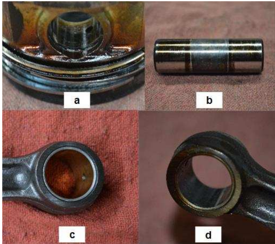
Figure 6-15. Photos of a) piston pin bore, b) piston pin, c) connecting rod pin bushing before testing, and d) connecting rod pin bushing after testing.
