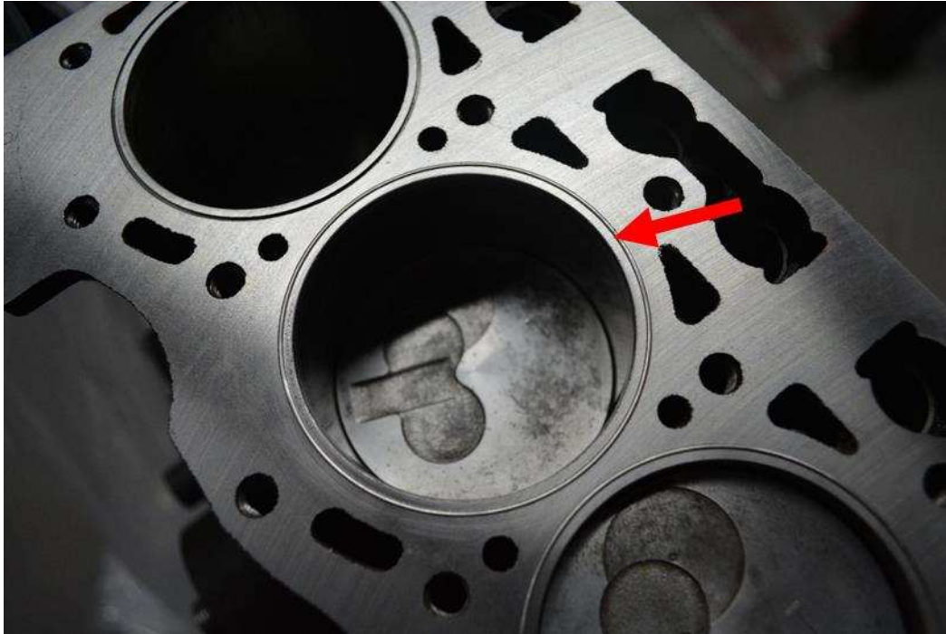
Figure 3-2. Engine block with stainless steel combustion chamber O-ring seals installed.
