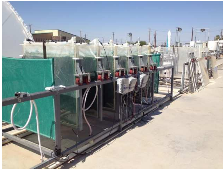
Figure 5: Picture of VFP array at AzCATI. The shading panels on the ends are to provide consistent conditions between all panels, eliminating exceptional irradiance for the end panels. Validation comparison was performed with interior panels only.
