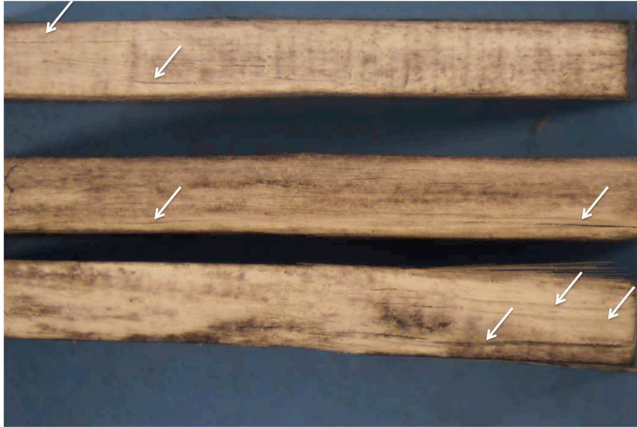
Figure 59: The damage incurred on CC(N) specimens from SBS testing. Arrows indicate lines that suggest shear failure.
