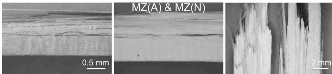
Figure 47: Typical damage in CC(N) composites as observed on the sides (left and center images) and fracture surfaces (far right image) of CC(N) specimens.
