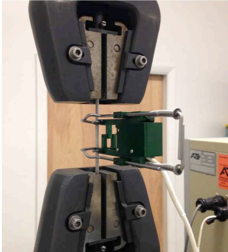
Figure 50: Typical configuration for tensile test of composite specimens.
