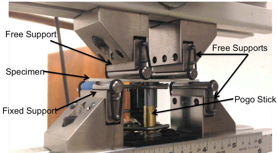
Figure 34. Fully articulating four-point flexure test fixture.
