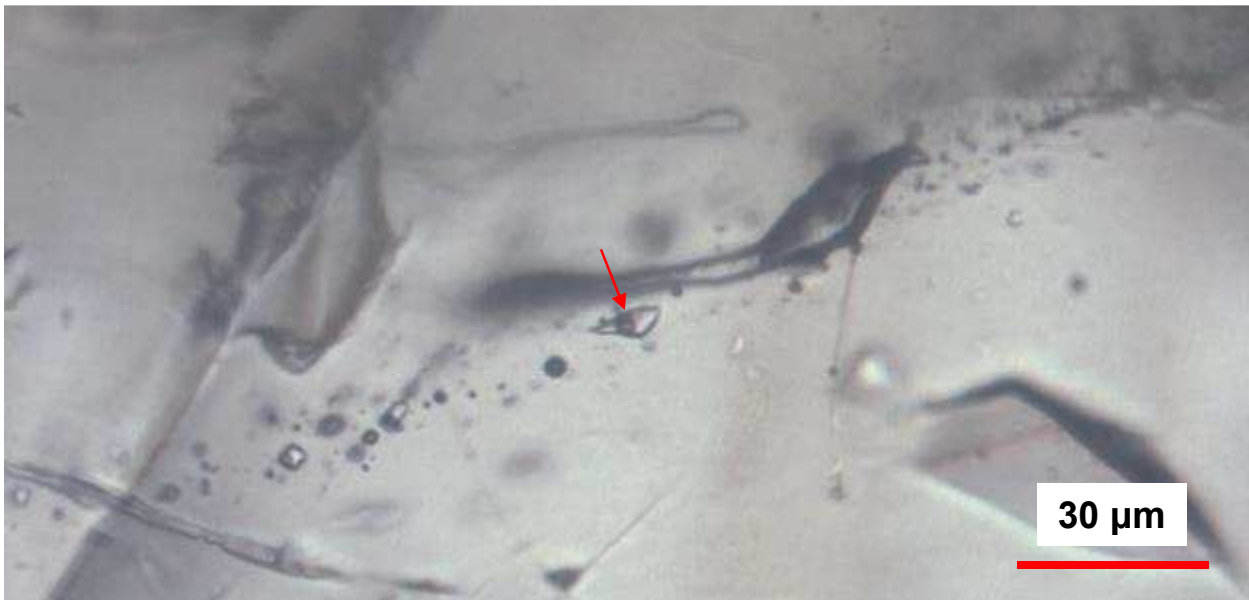
Figure 3.44. Figure showing three two-phase L-V fluid inclusions within an FIA, along an FIP. The inclusion in the center (red arrow) is elongated along the FIP. Sample AK111-1A.
