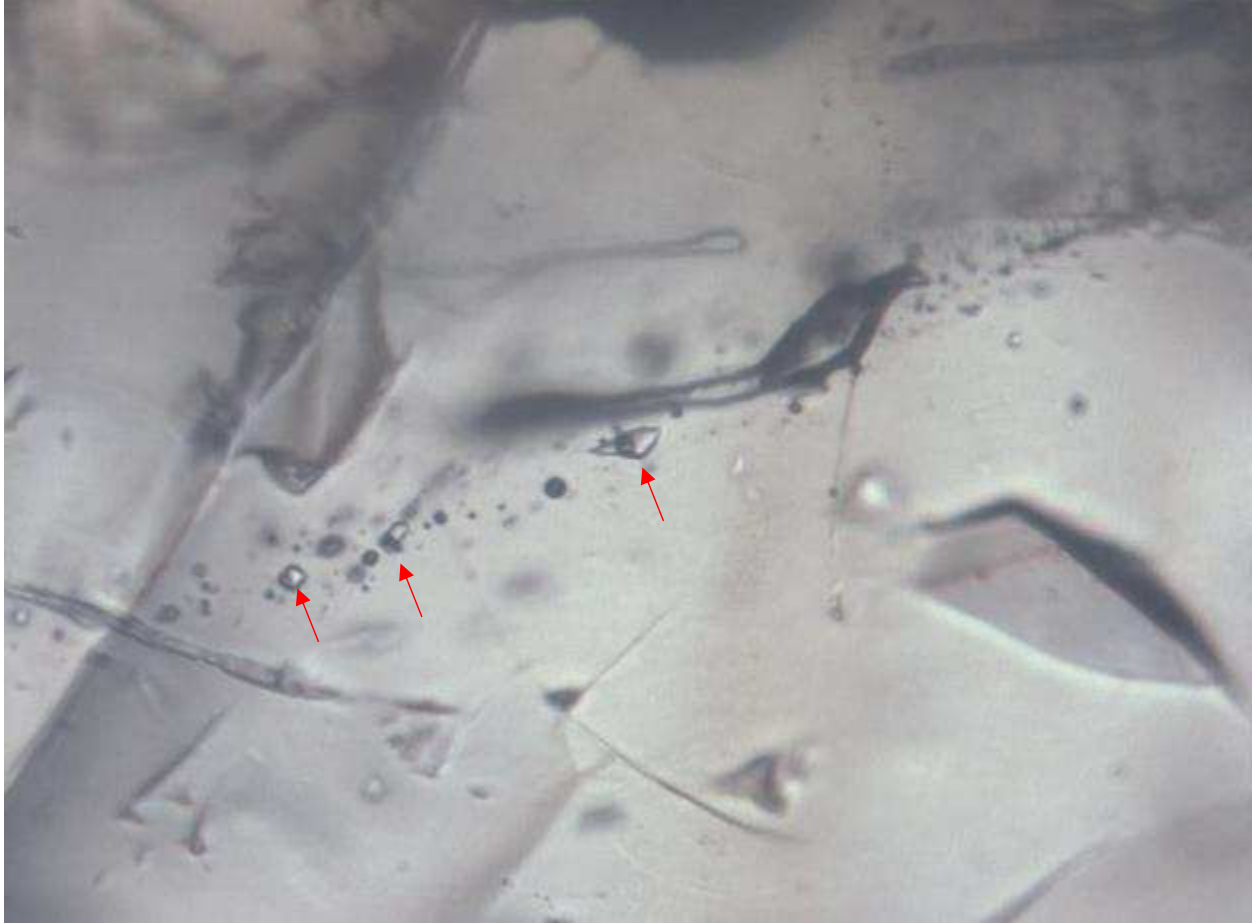
Figure 2.4. A typical fluid inclusion assemblage adjacent to the faults in the FCS, consisting of three liquid-vapor fluid inclusions (red arrows) aligned along one fluid inclusion plane. Thermometry measurements for all three inclusions were within 2°C of one another, suggesting they are temporally related and formed during the same “fluid event” (Bodnar, 2003).
