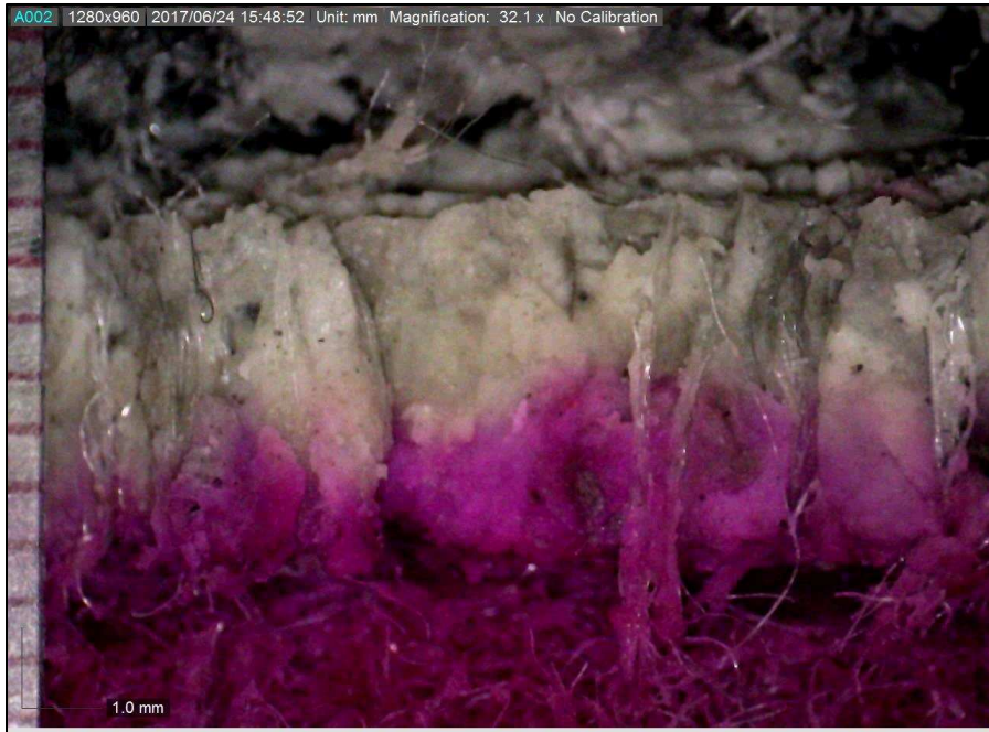
Figure F.37. Test 27a, DN9-B1. Snapped cross section. Similar staining of fiber bundle and clay portion, demonstrating possible less preferential flow in this portion of the GCL.
