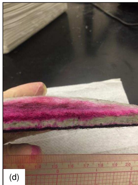
Figure F.4. Test 4a dyed disassembly, (a) view of influent side of GCL, (b) GCL cross section, (c) GCL cross section, (d) GCL cross section.
