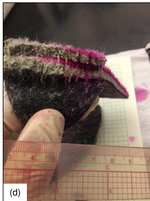
Figure F.5. Test 4a dyed disassembly, (a) GCL cross section, (b) GCL cross section, (c) GCL cross section, view of fiber bundles, (d) GCL cross section, view of fiber bundles.
