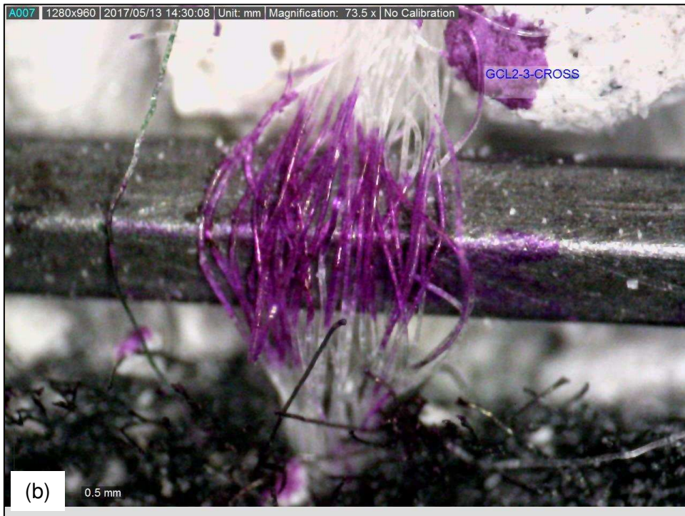
Figure B.26. Fiber bundle sample GCL2-3-CROSS. (a) Determination of the fiber bundle thickness. (b) Determination of the number of monofilament fibers per fiber bundle.
