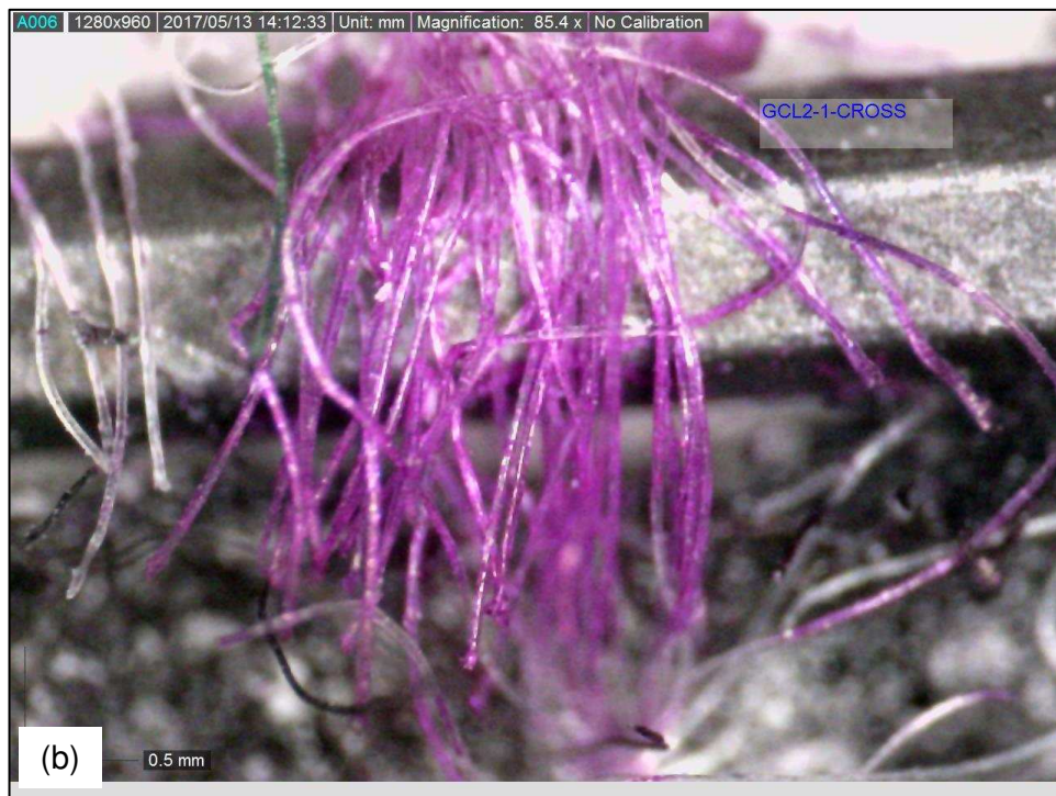
Figure B.22. Fiber bundle sample GCL2-1-CROSS. (a) Determination of the fiber bundle thickness. (b) Determination of the number of monofilament fibers per fiber bundle.
