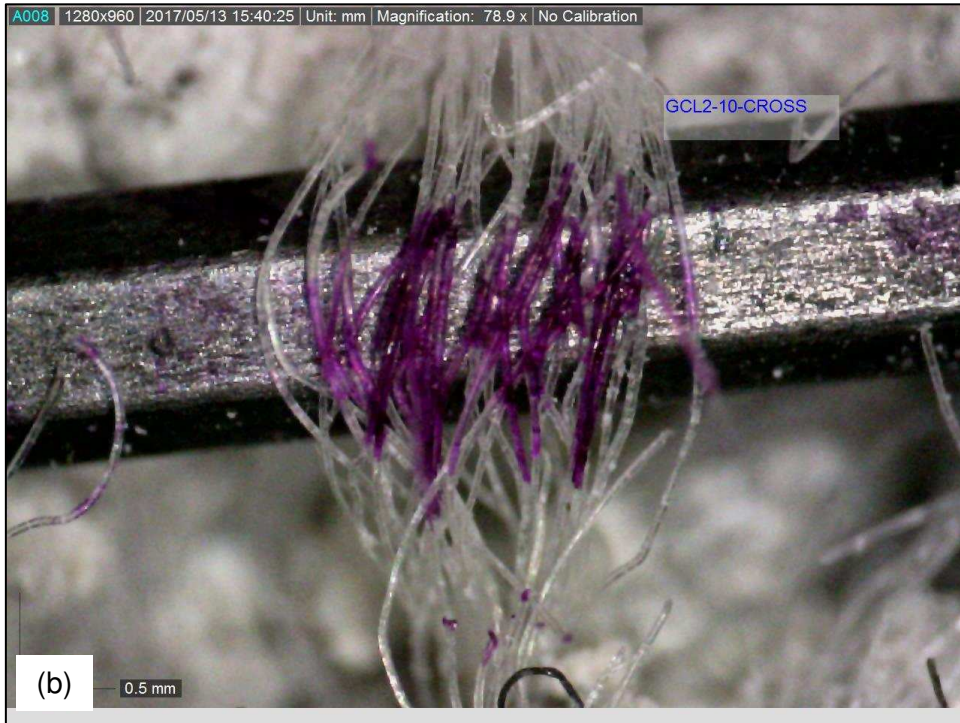
Figure B.40. Fiber bundle sample GCL2-10-CROSS. (a) Determination of the fiber bundle thickness. (b) Determination of the number of monofilament fibers per fiber bundle.
