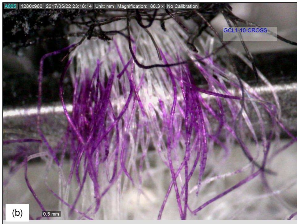
Figure B.20. Fiber bundle sample GCL1-10-CROSS. (a) Determination of the fiber bundle thickness. (b) Determination of the number of monofilament fibers per fiber bundle.
