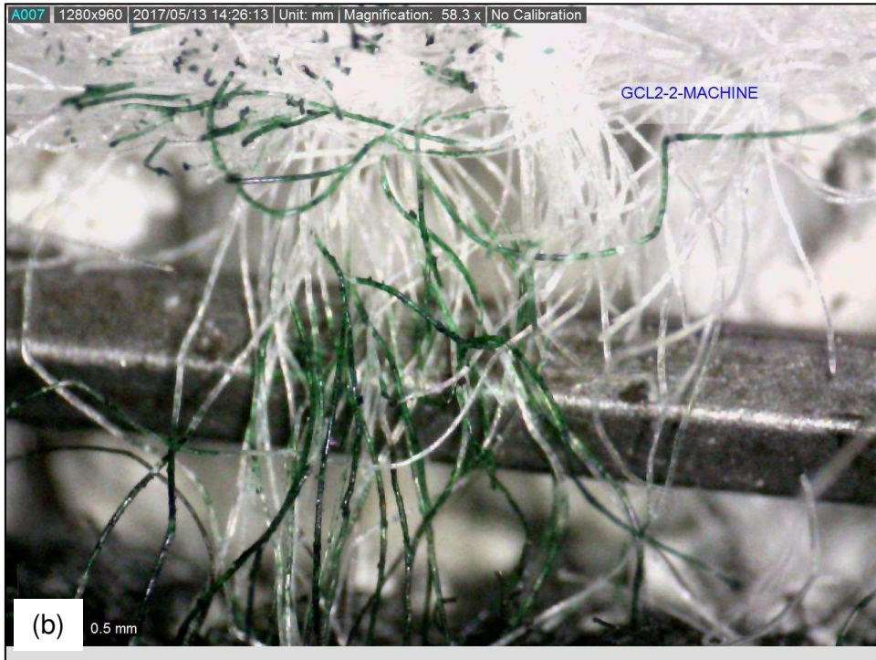
Figure B.23. Fiber bundle sample GCL2-2-MACHINE. (a) Determination of the fiber bundle thickness. (b) Determination of the number of monofilament fibers per fiber bundle.
