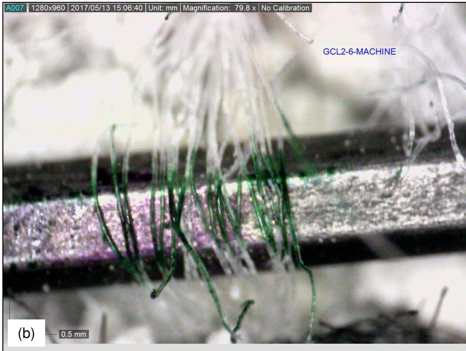
Figure B.31. Fiber bundle sample GCL2-6-MACHINE. (a) Determination of the fiber bundle thickness. (b) Determination of the number of monofilament fibers per fiber bundle.
