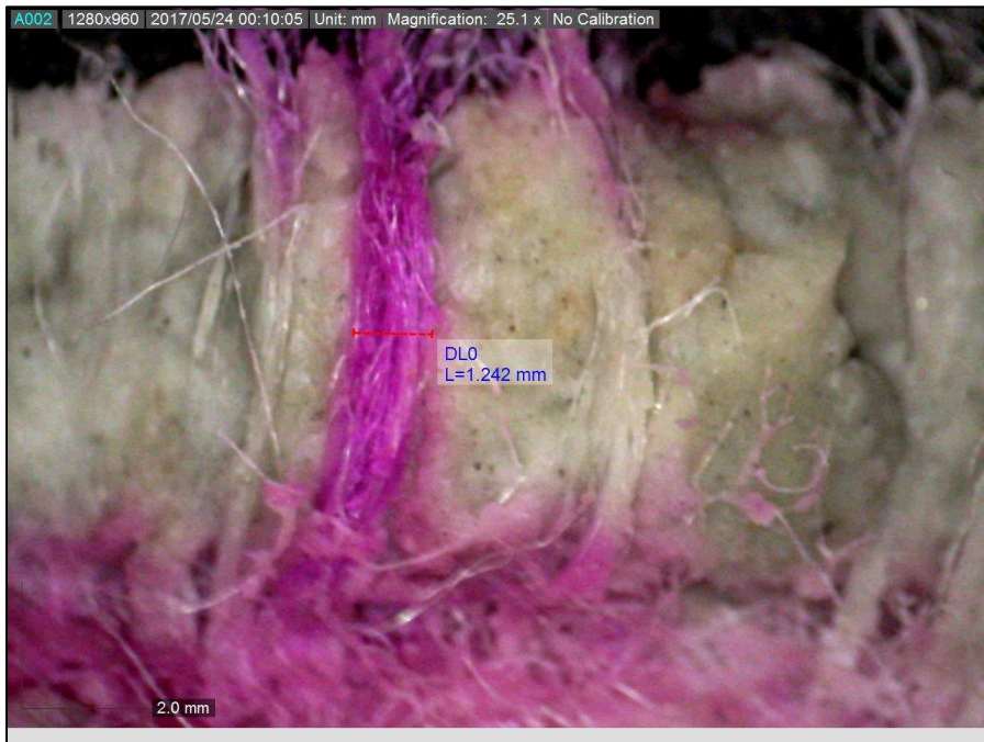
Figure F.56. Test 11c, DN9-L3. Snapped cross-section. Stained fiber bundle (middle). Unstained fiber bundles (left and right).
