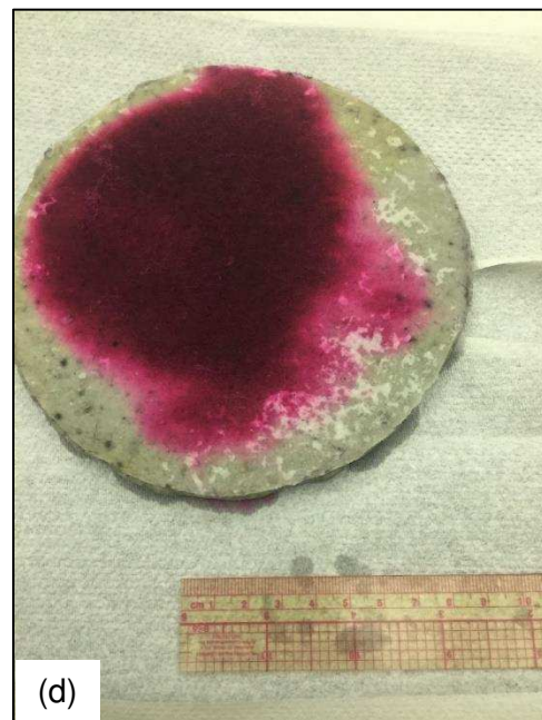
Figure F.3. Test 4a dyed disassembly, (a) top view of effluent geotextile, (b) bottom view of effluent filter paper, (c) bottom view of influent geotextile, (d) view of influent side of GCL.
