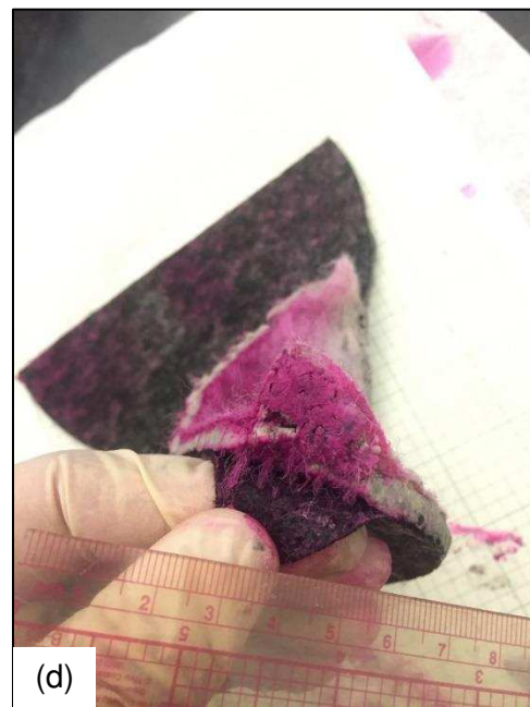
Figure F.6. Test 4a dyed disassembly, (a), (b), (c), (d) GCL cross section, view of fiber bundles.
