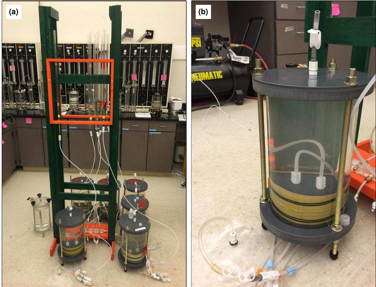
Figure 3.5. Photographs of (a) assembled mine-waste-leachate resistant permeameter assembly using gravity head method and (b) permeameter closeup.
