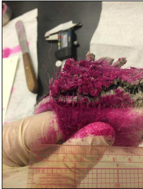
Figure F.8. Test 4a dyed disassembly. GCL cross section, view of fiber bundles.
