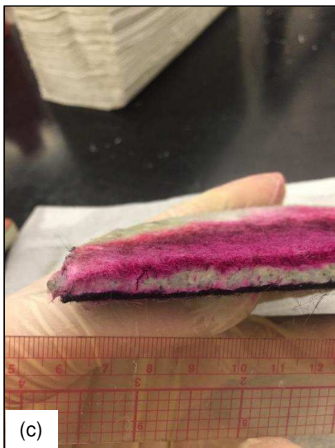
Figure F.4. Test 4a dyed disassembly, (a) view of influent side of GCL, (b) GCL cross section, (c) GCL cross section, (d) GCL cross section.
