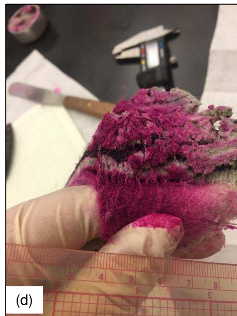
Figure F.7. Test 4a dyed disassembly, (a), (b), (c), (d) GCL cross section, view of fiber bundles.
