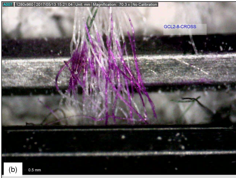
Figure B.36. Fiber bundle sample GCL2-8-CROSS. (a) Determination of the fiber bundle thickness. (b) Determination of the number of monofilament fibers per fiber bundle.
