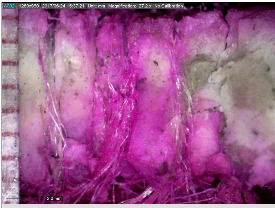
Figure F.36. Test 27a, DN9-B1. Stained fiber bundle demonstrating preferential flow, zoomed in.
