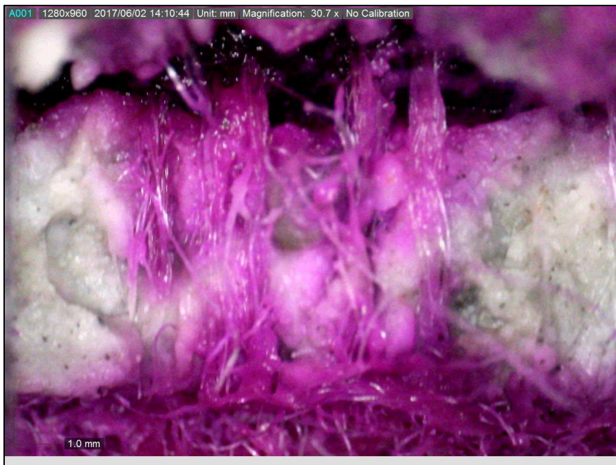
Figure F.46. Test 26a, DN9-G1. Snapped cross-section. Adjacent stained fiber bundles.
