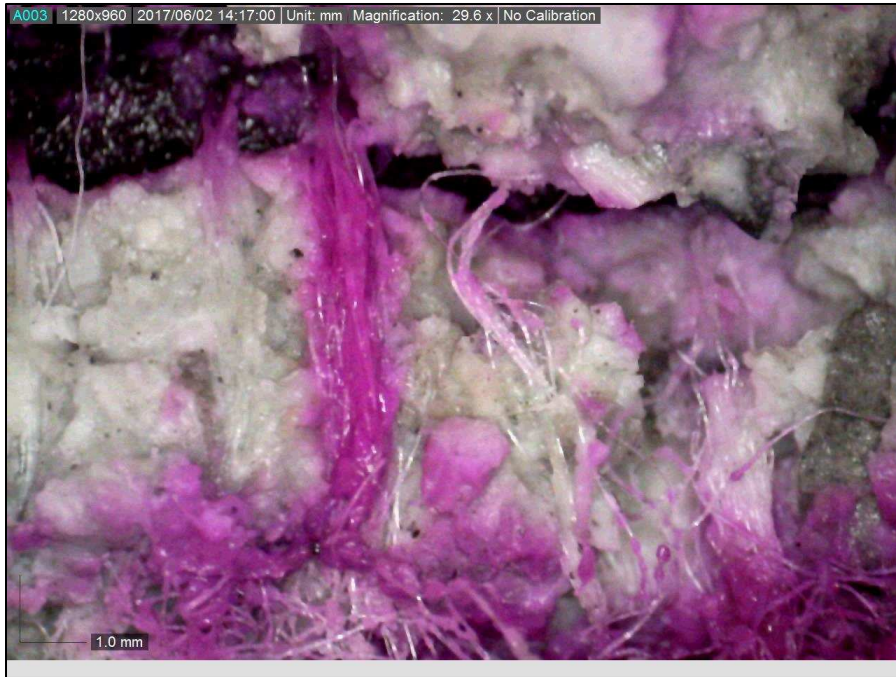
Figure F.47. Test 26a, DN9-G1. Snapped cross-section. Stained fiber bundle (middle) and unstained fiber bundles (left and right).
