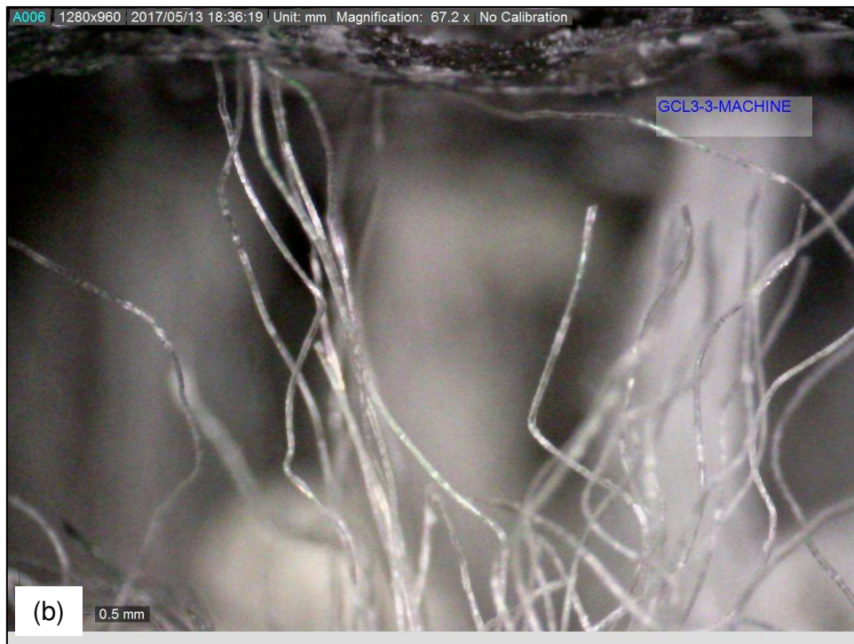
Figure B.45. Fiber bundle sample GCL3-3-MACHINE. (a) Determination of the fiber bundle thickness. (b) Determination of the number of monofilament fibers per fiber bundle.
