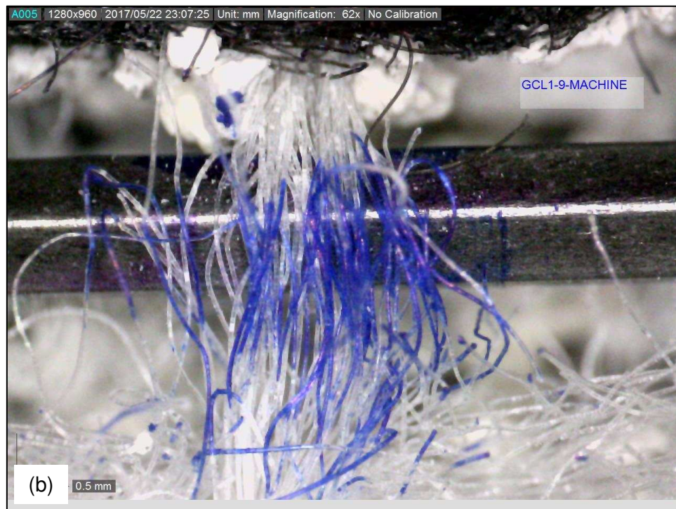
Figure B.17. Fiber bundle sample GCL1-9-MACHINE. (a) Determination of the fiber bundle thickness. (b) Determination of the number of monofilament fibers per fiber bundle.
