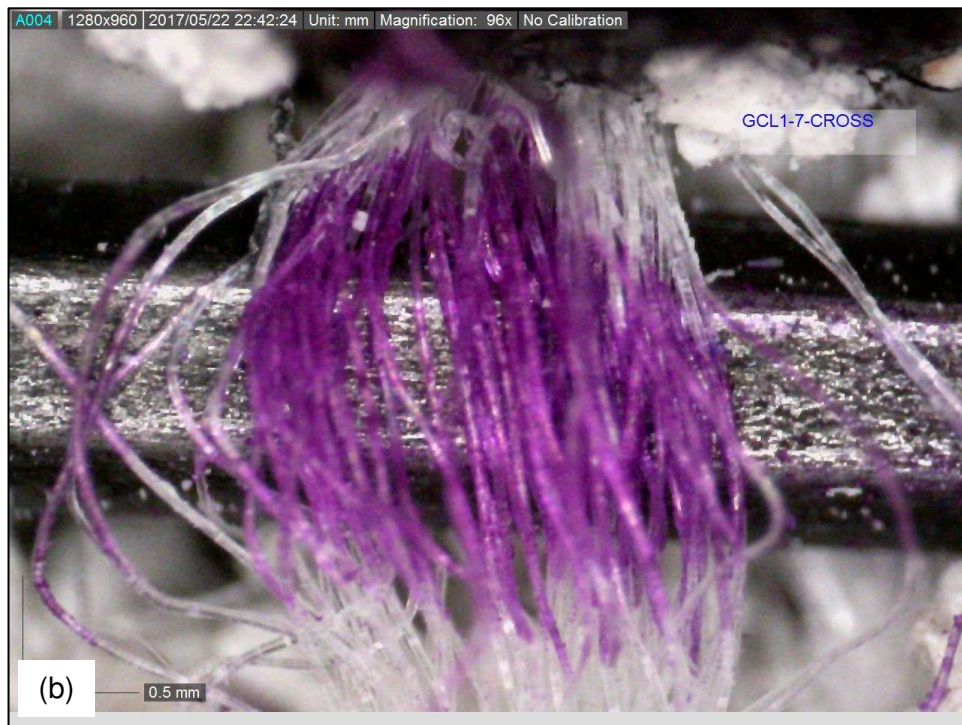
Figure B.14. Fiber bundle sample GCL1-7-CROSS. (a) Determination of the fiber bundle thickness. (b) Determination of the number of monofilament fibers per fiber bundle.
