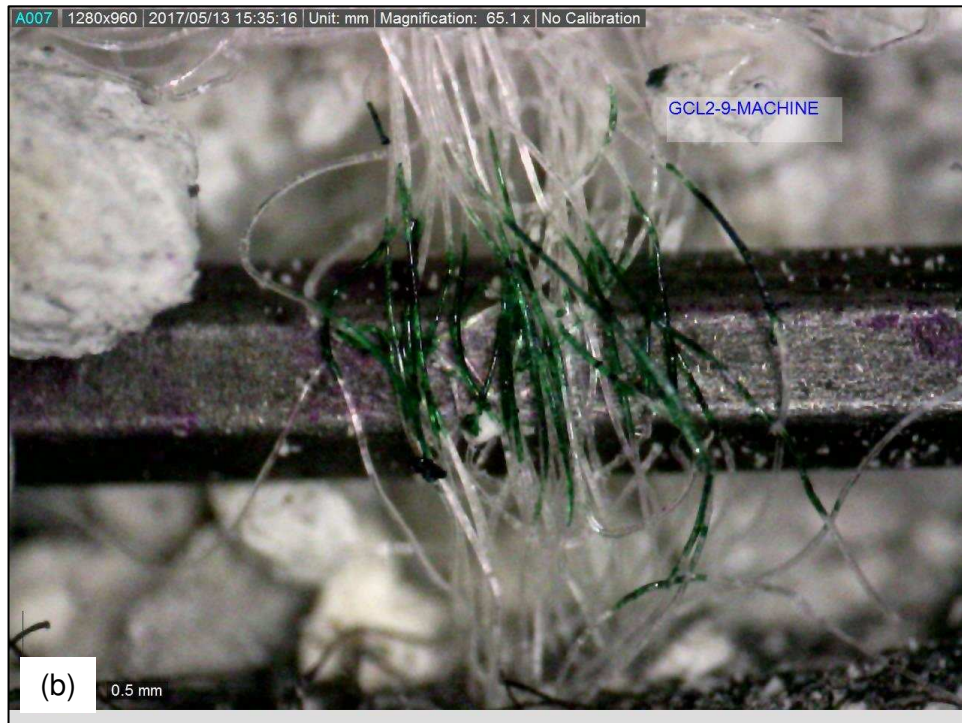
Figure B.37. Fiber bundle sample GCL2-9-MACHINE. (a) Determination of the fiber bundle thickness. (b) Determination of the number of monofilament fibers per fiber bundle.
