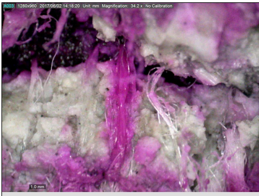
Figure F.48. Test 26a, DN9-G1. Snapped cross-section. Stained fiber bundle (middle) and unstained fiber bundles (left and right). Zoomed in.
