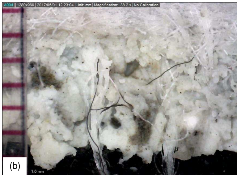
Figure 3.10. (a) Bentonite removed from GCL-2 permeated with synthetic copper mining process solution (Cu-PS). (b) GCL-2 cross-section permeated with Cu-PS.
