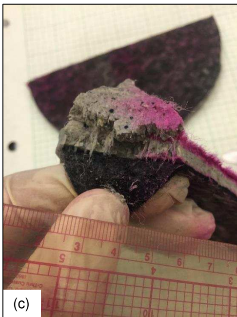
Figure F.5. Test 4a dyed disassembly, (a) GCL cross section, (b) GCL cross section, (c) GCL cross section, view of fiber bundles, (d) GCL cross section, view of fiber bundles.
