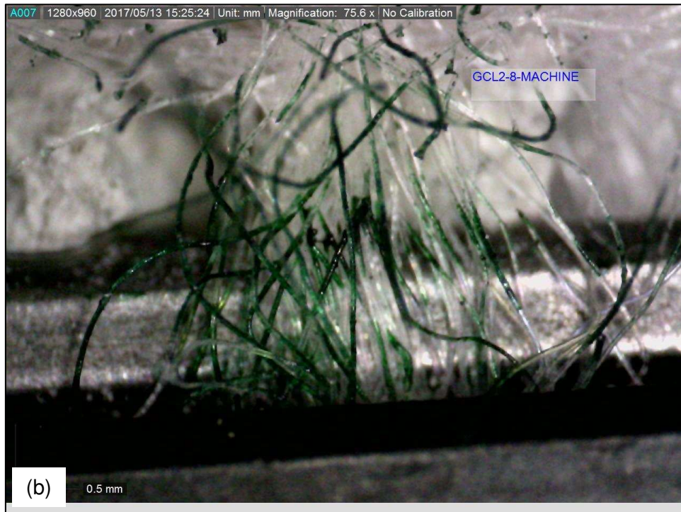
Figure B.35. Fiber bundle sample GCL2-8-MACHINE. (a) Determination of the fiber bundle thickness. (b) Determination of the number of monofilament fibers per fiber bundle.
