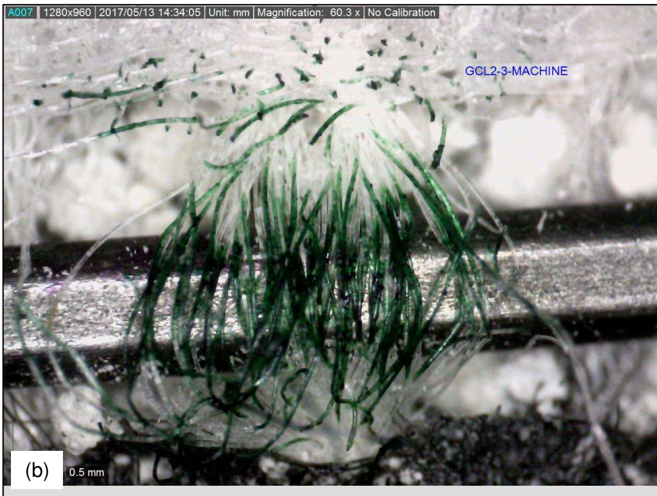
Figure B.25. Fiber bundle sample GCL2-3-MACHINE. (a) Determination of the fiber bundle thickness. (b) Determination of the number of monofilament fibers per fiber bundle.
