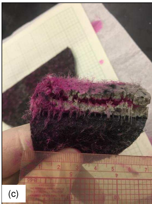
Figure F.7. Test 4a dyed disassembly, (a), (b), (c), (d) GCL cross section, view of fiber bundles.
