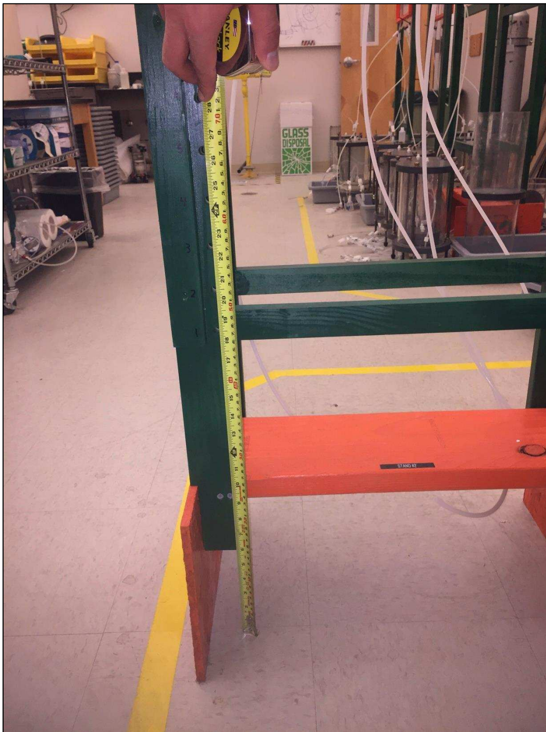
Figure C.1. Measurement of variable a , the distance from floor to the first pinhole measured in cm.
