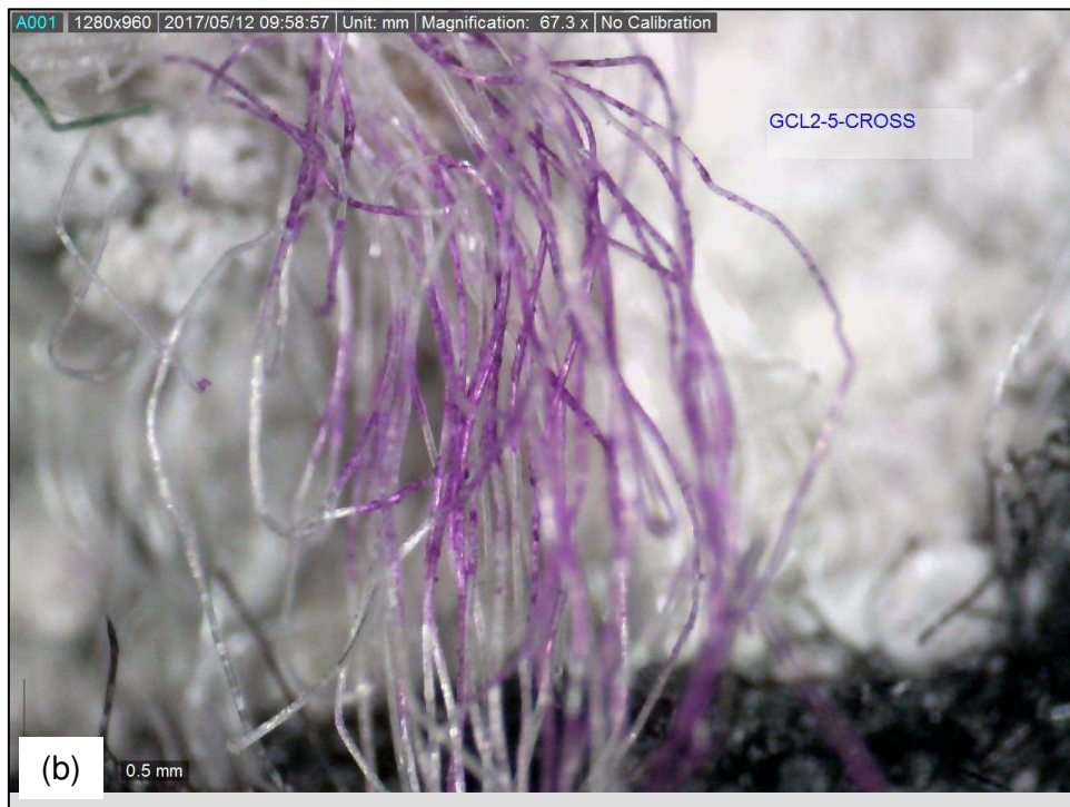
Figure B.30. Fiber bundle sample GCL2-5-CROSS. (a) Determination of the fiber bundle thickness. (b) Determination of the number of monofilament fibers per fiber bundle.
