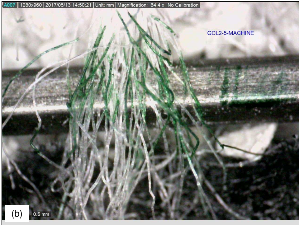
Figure B.29. Fiber bundle sample GCL2-5-MACHINE. (a) Determination of the fiber bundle thickness. (b) Determination of the number of monofilament fibers per fiber bundle.
