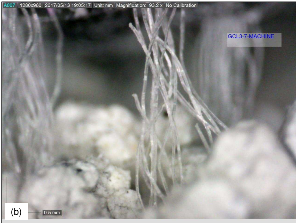
Figure B.53. Fiber bundle sample GCL3-7-MACHINE. (a) Determination of the fiber bundle thickness. (b) Determination of the number of monofilament fibers per fiber bundle.
