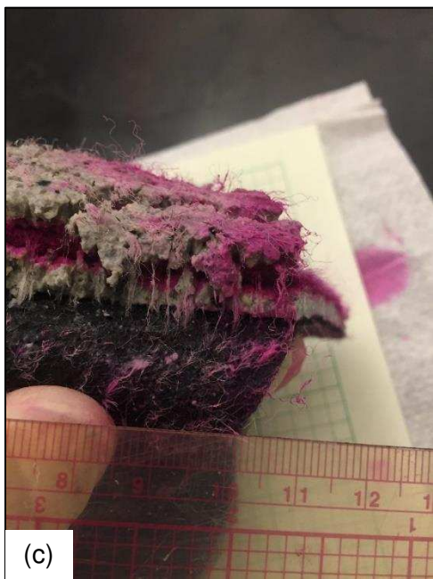
Figure F.6. Test 4a dyed disassembly, (a), (b), (c), (d) GCL cross section, view of fiber bundles.
