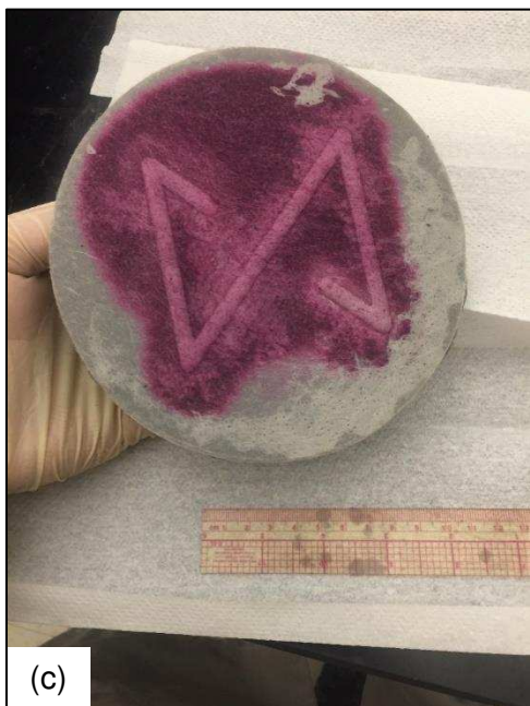
Figure F.3. Test 4a dyed disassembly, (a) top view of effluent geotextile, (b) bottom view of effluent filter paper, (c) bottom view of influent geotextile, (d) view of influent side of GCL.
