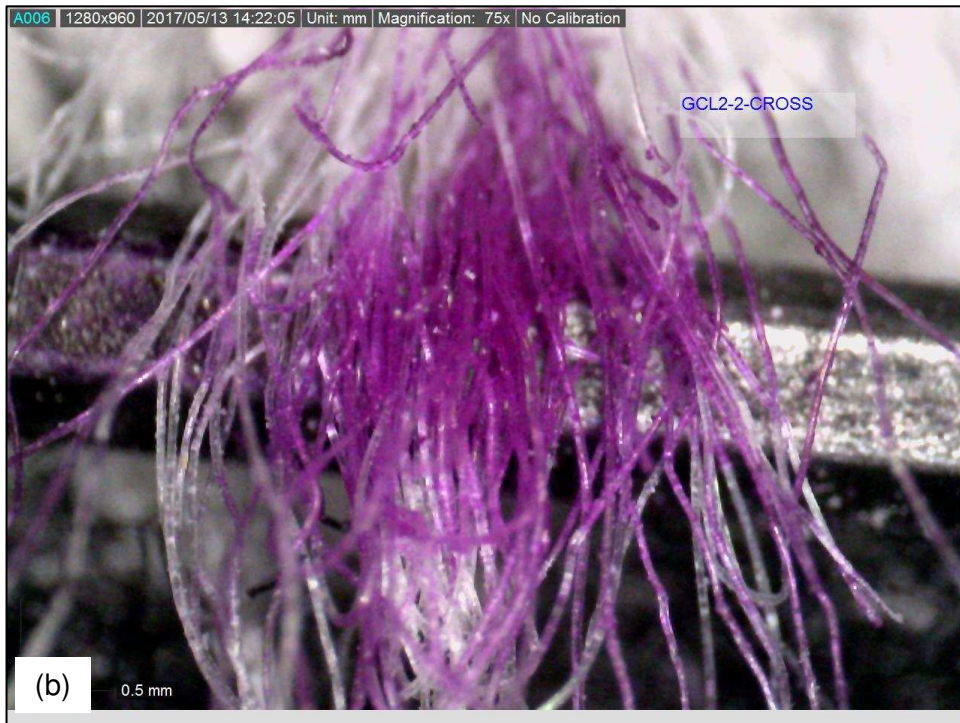
Figure B.24. Fiber bundle sample GCL2-2-CROSS. (a) Determination of the fiber bundle thickness. (b) Determination of the number of monofilament fibers per fiber bundle.
