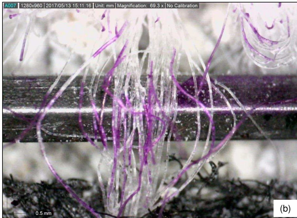
Figure 2.4. Exemplary photograph for (a) measuring fiber bundle thickness and (b) counting the number of monofilament fibers per fiber bundle using a digital stereoscopic microscope.
