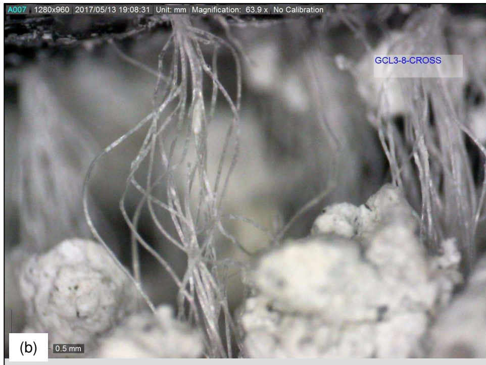
Figure B.56. Fiber bundle sample GCL3-8-CROSS. (a) Determination of the fiber bundle thickness. (b) Determination of the number of monofilament fibers per fiber bundle.
